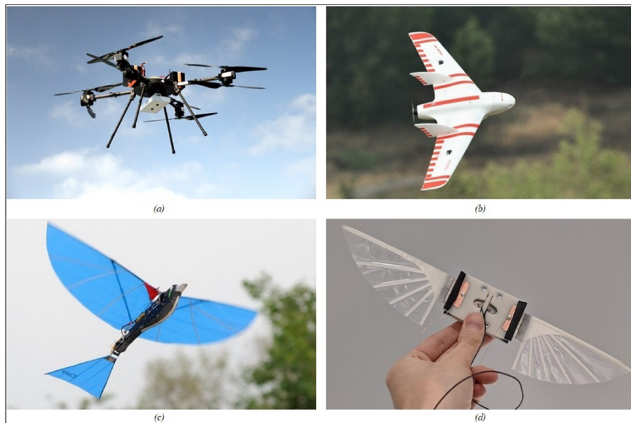
Figure 2.7: Different types of UAVs (a) rotary-wing, (b) fixed-wing (c) flapping-wing (Ornithopters) (d) flapping-wing (Entomopters).
