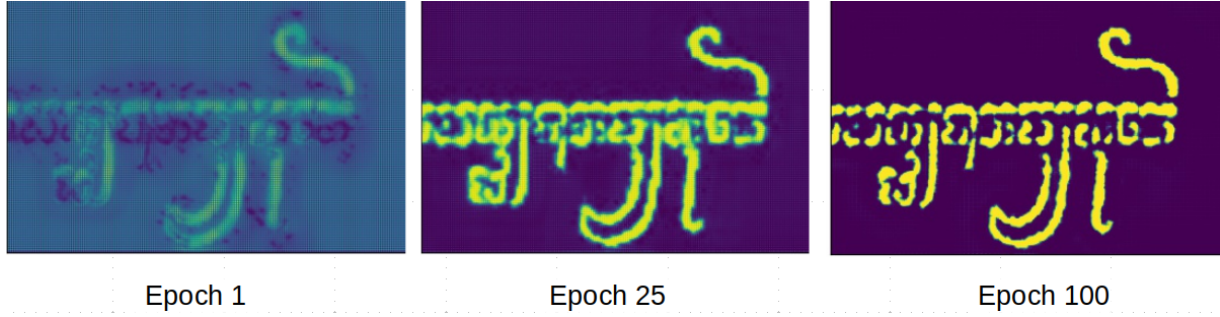
Figure 4.9: Evolution of confidence score. Bright pixels have a high score, dark ones have a low score.
