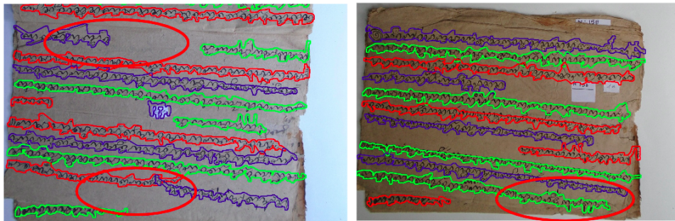
Figure 5.26: Cases where the lines are considered to split into two segments. (Left) correct segmentation, the lines are split into two distinct lines (at the red circle). (Right) wrong segmentation, the line has to be split into two lines.
