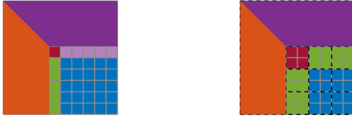
Figure 2.12: GETRF algorithm at a given step where the orange panel is the factorized L matrix, the purple panel is the factorized U matrix, the red element (resp. blocks) corresponds to the factorization step, the green elements (resp. blocks) correspond to the solve step and the blue elements (resp. blocks) correspond to the update step. Left: Element-wise factorization. Right: Block-wise factorization.
