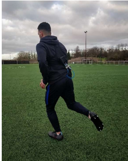
Figure 3. Outdoor football field used in this study and data acquisition system (MaxiPhyling, Phyling, France) connected to each shoe by a wire and worn by subjects in a lightweight sport vest.
