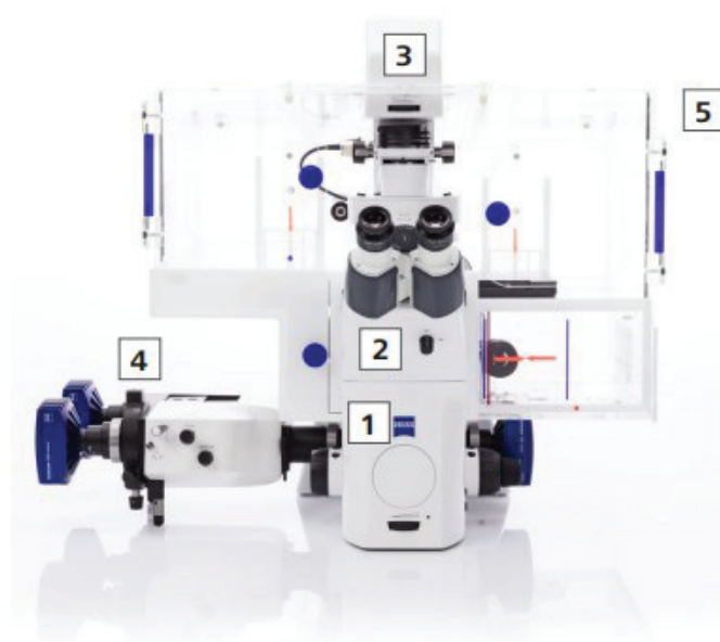
Figure 2.27: Axio Observer microscope 7 by Zeiss showing 1) the microscope 2) Objectives are within the microscope 3) Illumination 4) imaging system and 5) Accessories if live cell imaging is needed.
