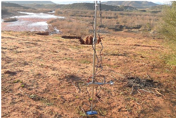
Photo 4-3 Micro-moulinet de type OTT (El Orfi, 2019)
