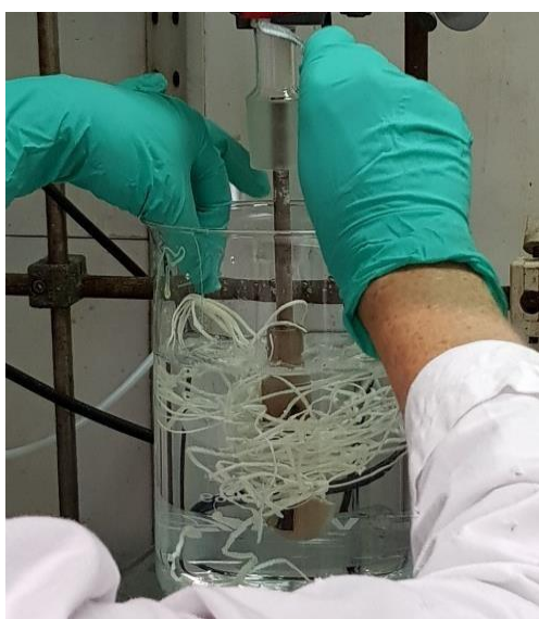
Figure II-19. P6 Fluorinated polythioether polymer precipitation in acidic medium (left) and P6 after drying
