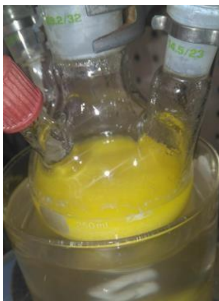
Figure III-17. Phosphonation using strategy 1 (conventional heating).
