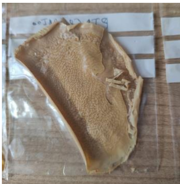
Figure IV-6. Film with phase separation after evaporation of the solvent.
