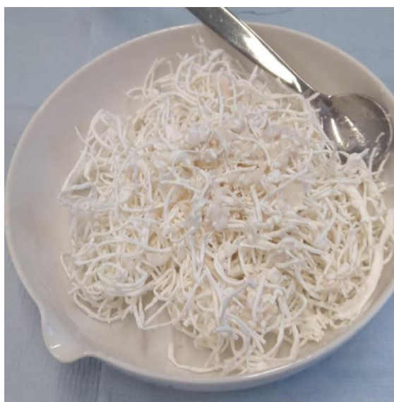
Figure II-19. P6 Fluorinated polythioether polymer precipitation in acidic medium (left) and P6 after drying
