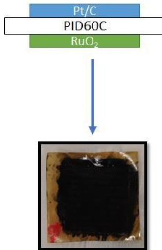
Figure IV-14. Membrane 3x3cm. P4SM-c_CCM after catalyst deposition.
