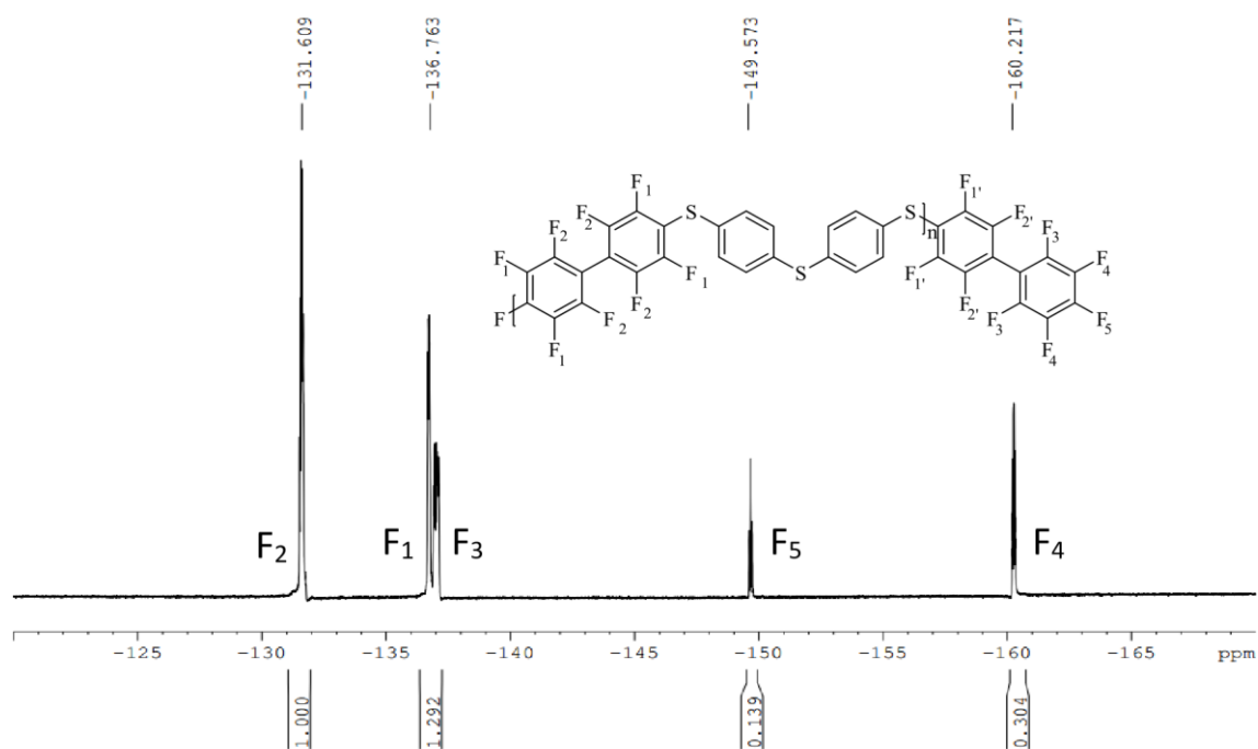
Figure II-26. ^{19}\text{F} NMR of polymerization of DCFB and TMSTB
