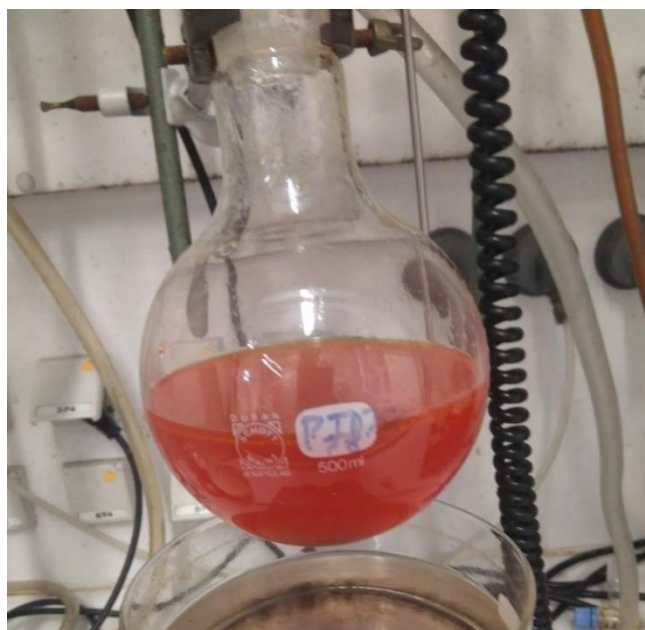
Figure III-34. Solution after sulfonating using \text{Na}_2\text{S}
