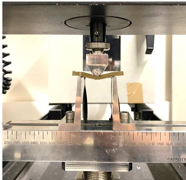
Figure 45: Instantaneous moment of performing the three-point bending test.
