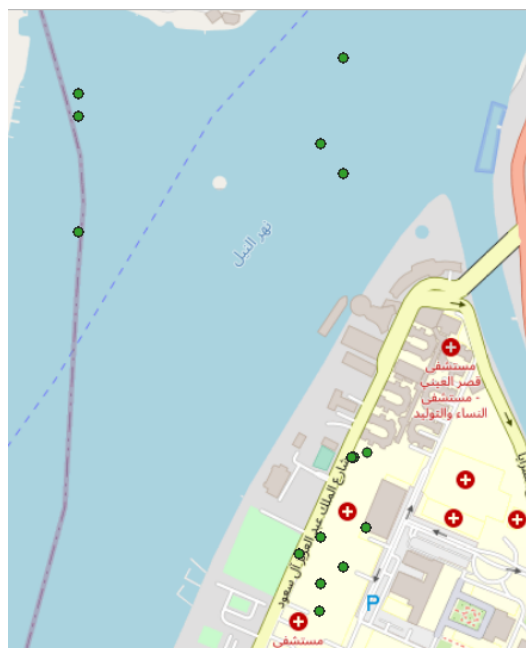
Figure 13. Representation of the cluster found as part of the event (5 tracks, 9418 points) in Cairo (Egypt) in August 2018 [47]. Note that 6309 points are affected by low GPS accuracy due to the measurement inside a building, which makes them poorly positioned on the Nile River; represented area of approximately 950 \text{ m} \times 820 \text{ m} . All the data are extracted from the NoiseCapture database [41].
