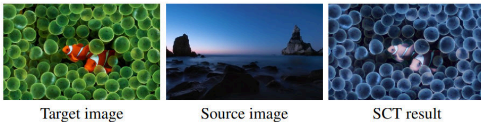
Figure 4.5: Example of color transfer using the method proposed by (Giraud et al., 2017). In color transfer, the inputs are the target and reference color images. The objective of this task is to apply the color palette of the source image to the target image while preserving the content and structure of the target image.
