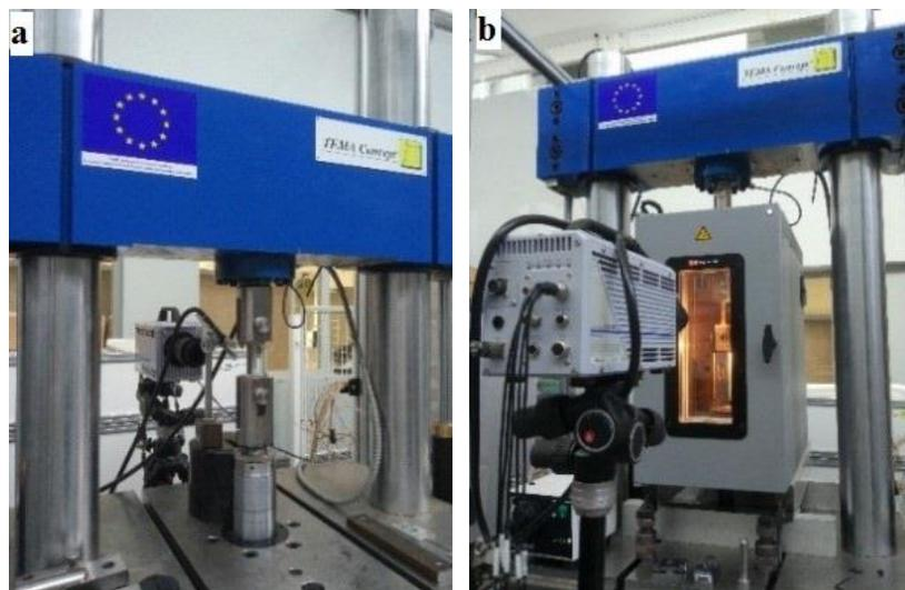
Fig. 2.2 (a) Servo-hydraulic tensile testing machine; (b) Insulated box.
