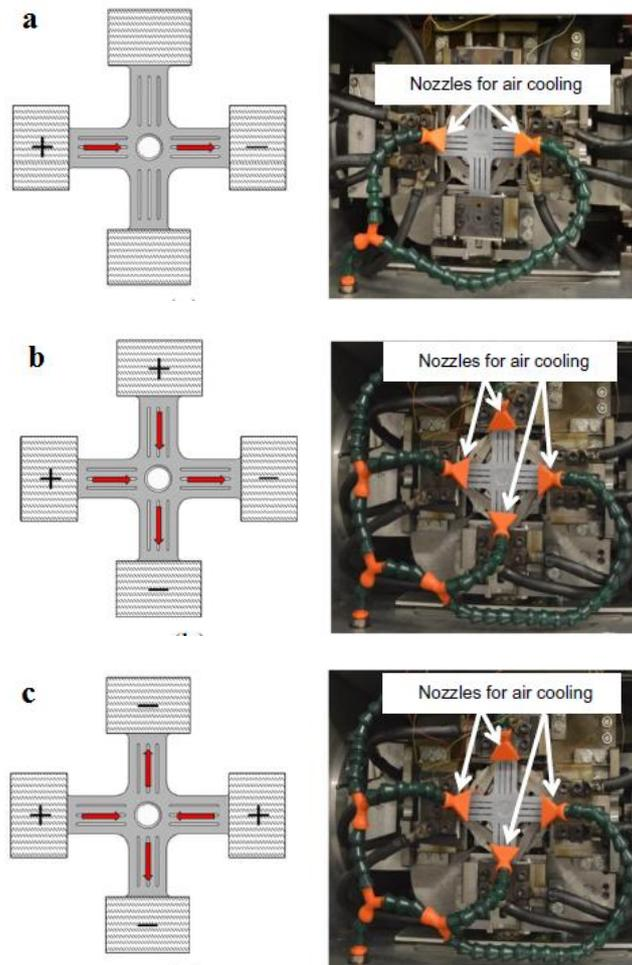
Fig. 1.30 Three strategies of specimen heating and cooling: (a) Type-1; (b) Type-2; (c) Type-3 (Arrows on specimens represent polarity of electrical potential). [105]
