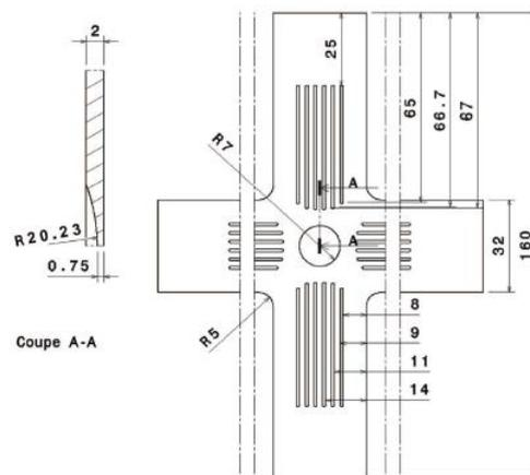
Fig. 1.22 Geometry of the cruciform specimen for Song. [97]
