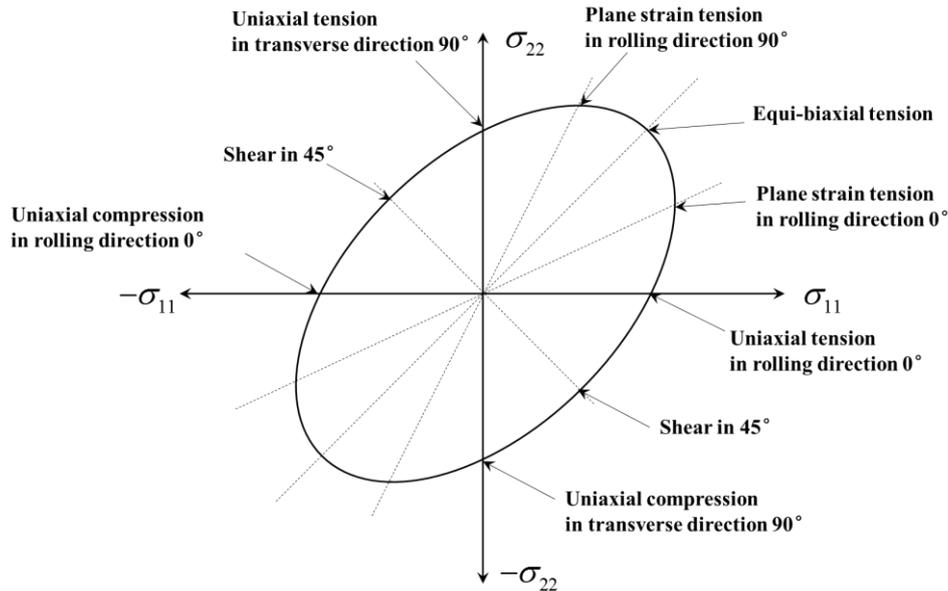
Fig. 1.1 Yield surface under plane stress condition.
