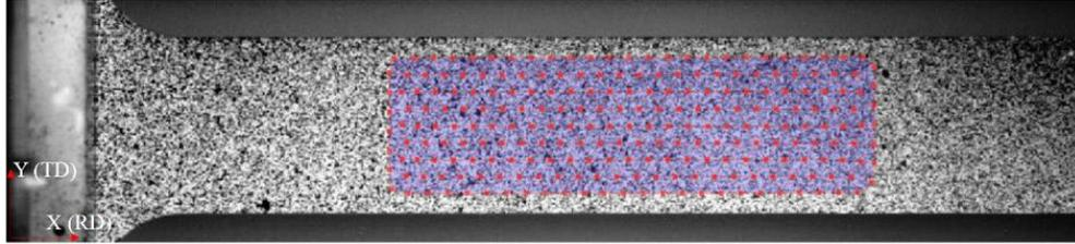
Fig. 2.3 Analyzed area of uniaxial tensile specimen.
