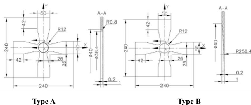
Fig. 1.20 Cruciform specimen with circular grooves. [95]
