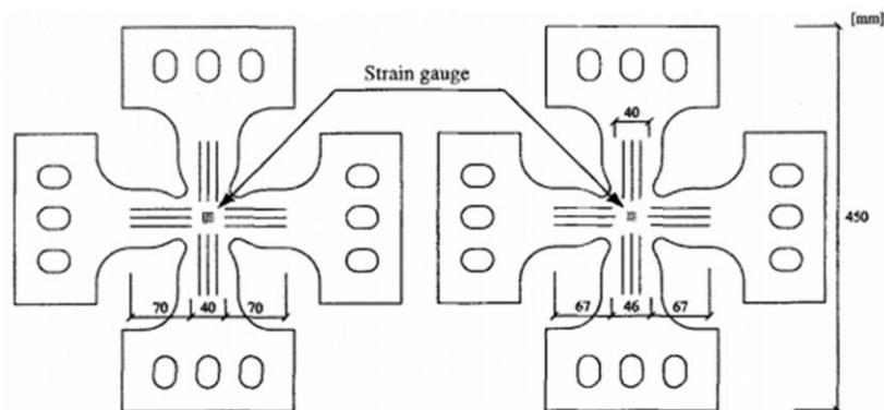
Fig. 1.18 Cruciform of the specimen for Gozzi. [93]
