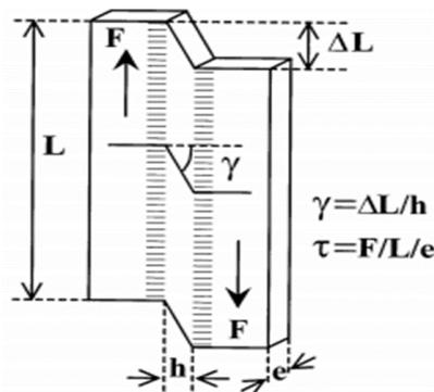
**Fig. 1.8 Shape of specimen in [64].**
