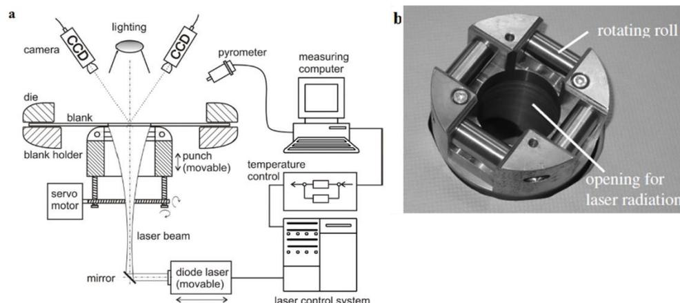
*Fig. 1.24 (a) Experimental setup; (b) Special designed hollow punch. [101]*
