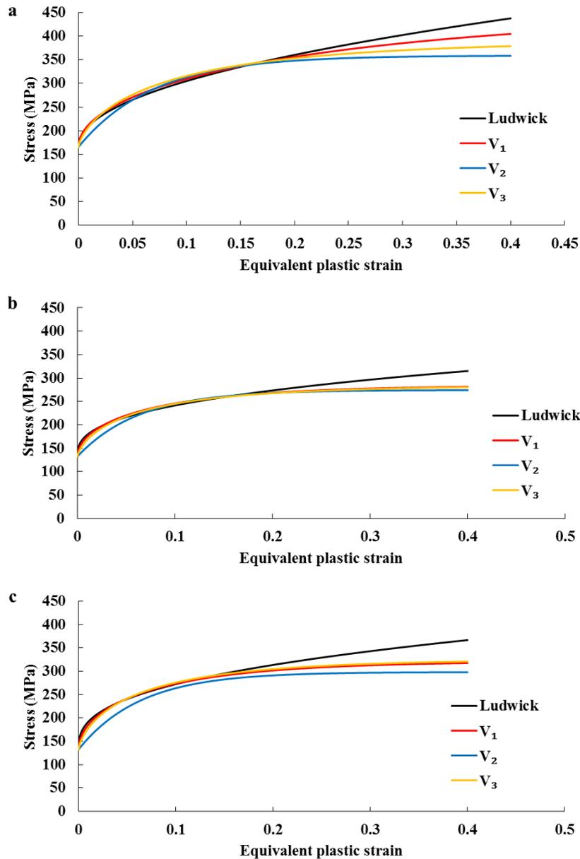
Fig. 2.15 Predictive results for Ludwick,  $V_1$ ,  $V_2$ , and  $V_3$  models with strain levels up to 40%:
