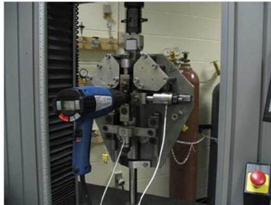
*Fig. 1.25 Biaxial testing device and heating gun [102].*
