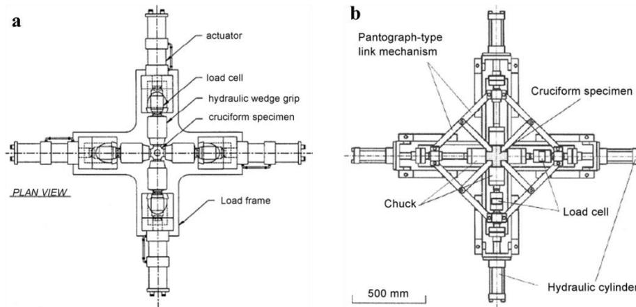
Fig. 1.12 Stand-alone biaxial testing machines: (a) Makinde 1992 [82]; (b) Kuwabara 1998 [83].
