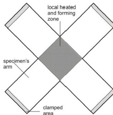
Fig. 1.23 Schematic design of the cruciform specimen. [101]
