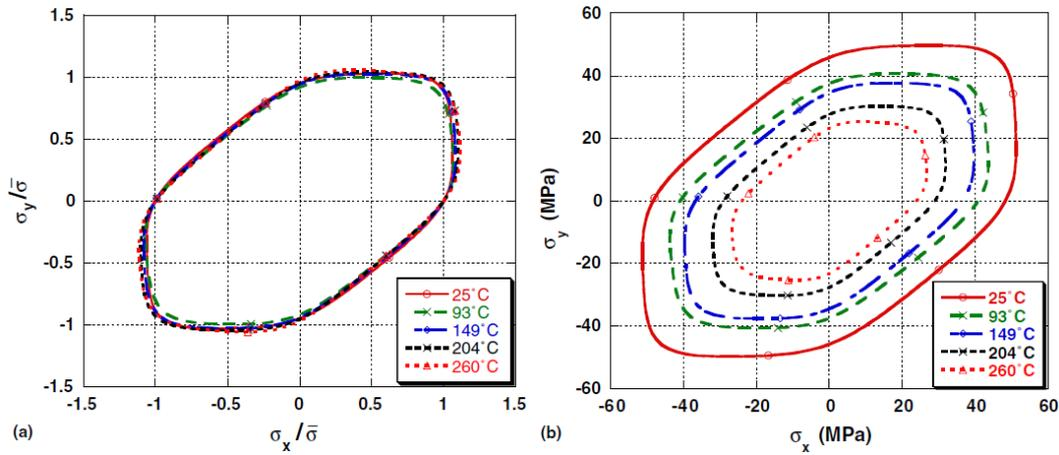
**Fig. 1.3** 2D-Plot of Barlat's yield function for AA3003-H111 at several elevated temperatures. (a) Stresses normalized with the flow stress to show the change in the yield surface shape. (b) Plot of actual stresses to show the change in the size of the yield surface. [18]
