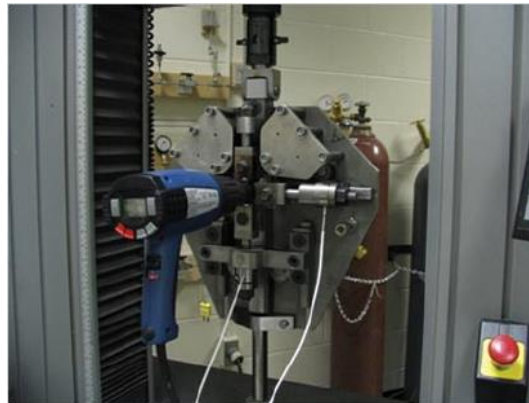
Fig. 1.25 Biaxial testing device and heating gun [102].
