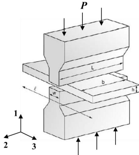
Fig. 1.9 Schematic diagram of plane strain compression test. [69]
