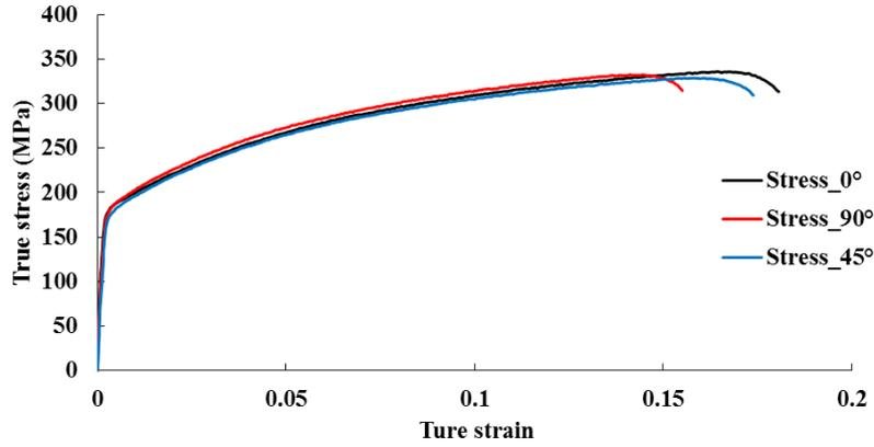
**Fig. 2.4 True stress-strain curves along the three directions.**
