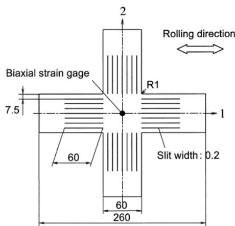
Fig. 1.14 Cruciform of specimen (Units are in mm) [87].
