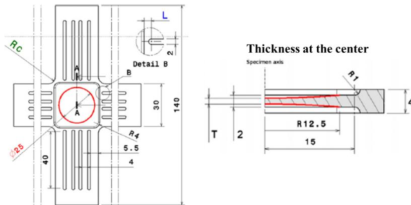
Fig. 1.21 Geometry of the cruciform specimen for Zidane. [96]
