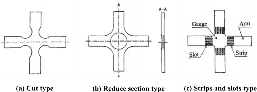
Fig. 1.13 Different type of cruciform specimen. [86]
