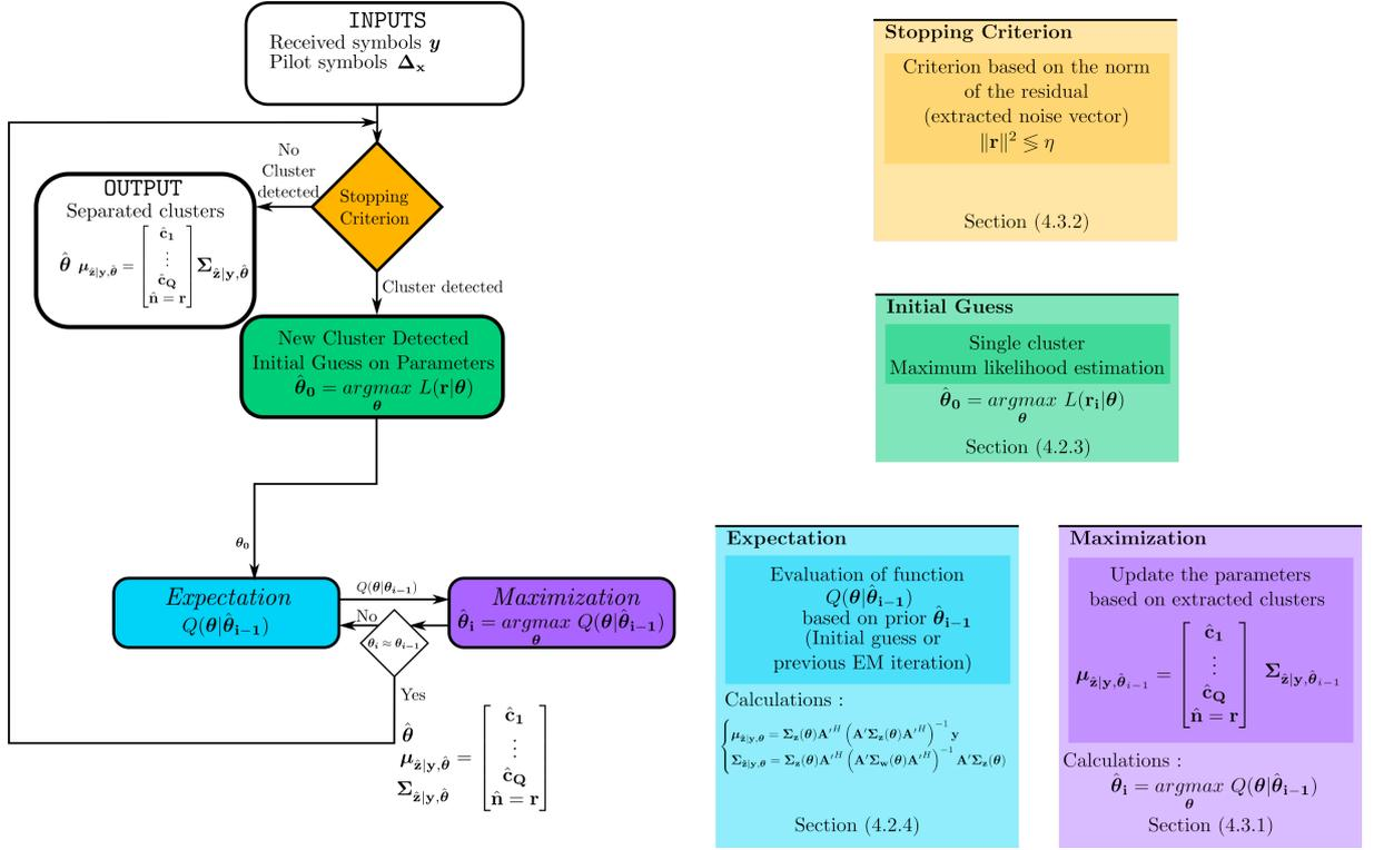
Figure 4.9 – Flowchart of the cluster separation and estimation procedure.
