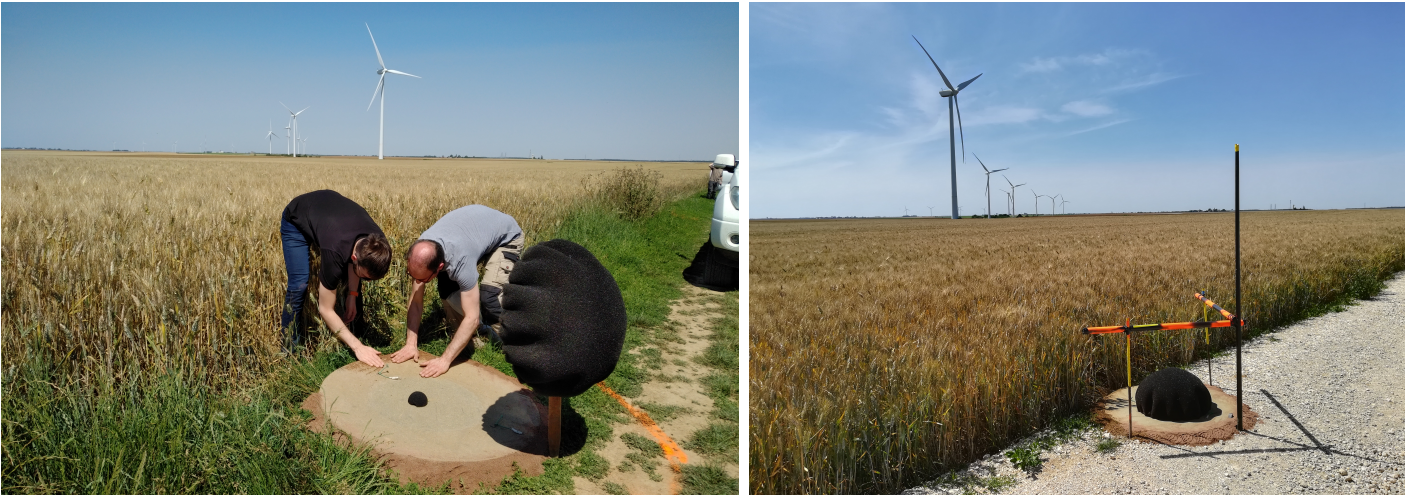
Figure 4.8: Left: The installation of the microphone at the IEC point on the ground in the centre of a circular reflective plate of 1m diameter. The installed wind screen of diameter 9cm can be seen. Right: The installed IEC point S3 with the wind screen of diameter 50cm.
