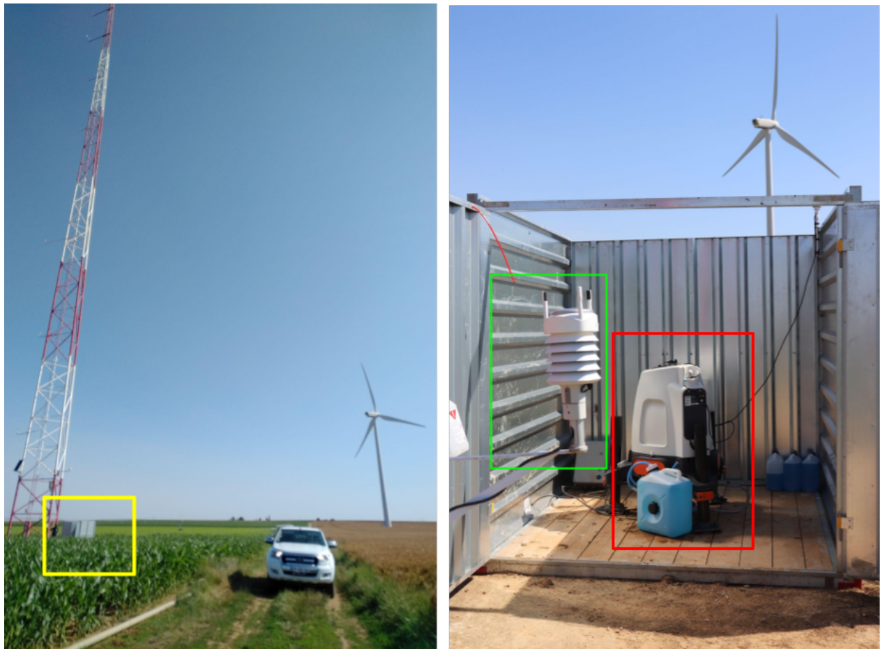
Figure 4.7: The meteorological mast with multiple sensors at different heights and the location of the LIDAR highlighted (left). The LIDAR (Zephir ZX300) in red focus, fitted with the local weather data logger in green focus (right).
