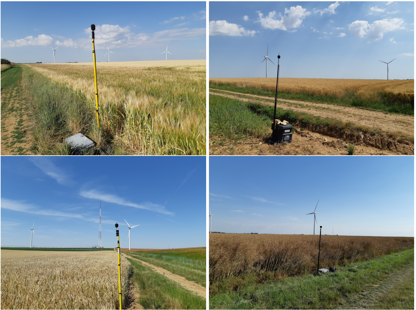
Figure 4.9: The installed sonometers at a height of 2m. The difference in the surrounding grounds can be clearly seen. From top left, clockwise: L1-N3, L2-S1, L3-S2, L4-N1.
