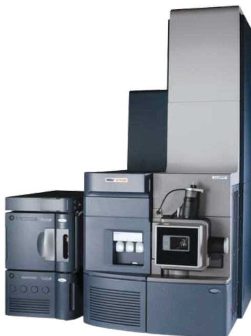
Figure 2. Ultra-performance high-resolution chromatography system coupled to a quadrupole time-of-flight (UPLC-QTOF) from Waters Corp.
