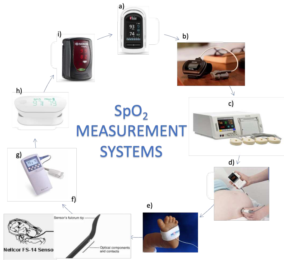
Figure 3-4 Examples of Commercial SpO 2 sensors on the market. a) Masimo MightySat b) Philips Respironics WristOx2 c) Philips Avalon Fetal Monitor d) Doppler foetal Sonicaid SR2 e) NeoPulse Pulse Oximeter f) OxiFirst™ FS14 Sensor g) Nellcor OxiMax N-65 Handheld Pulse Oximeter h) iHealth Air Wireless i) Nonin Onyx Vantage 9590.
