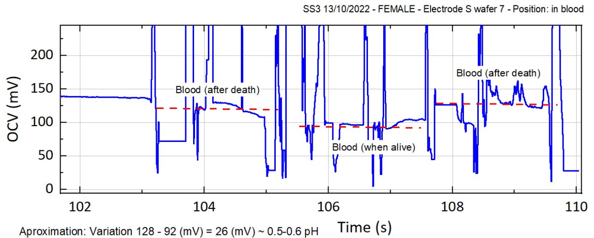
Figure 2-73 OCV signal recorded by flexible pH probe in mouse's blood. Average level of variation is obtained by subtracting the parasitic noise due to manipulation.
