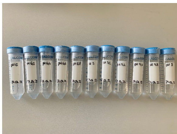
Figure 2-24 Test solution PBS at different pH levels.
