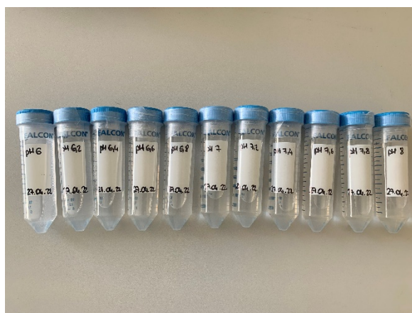
Figure 2-24 Test solution PBS at different pH levels.
