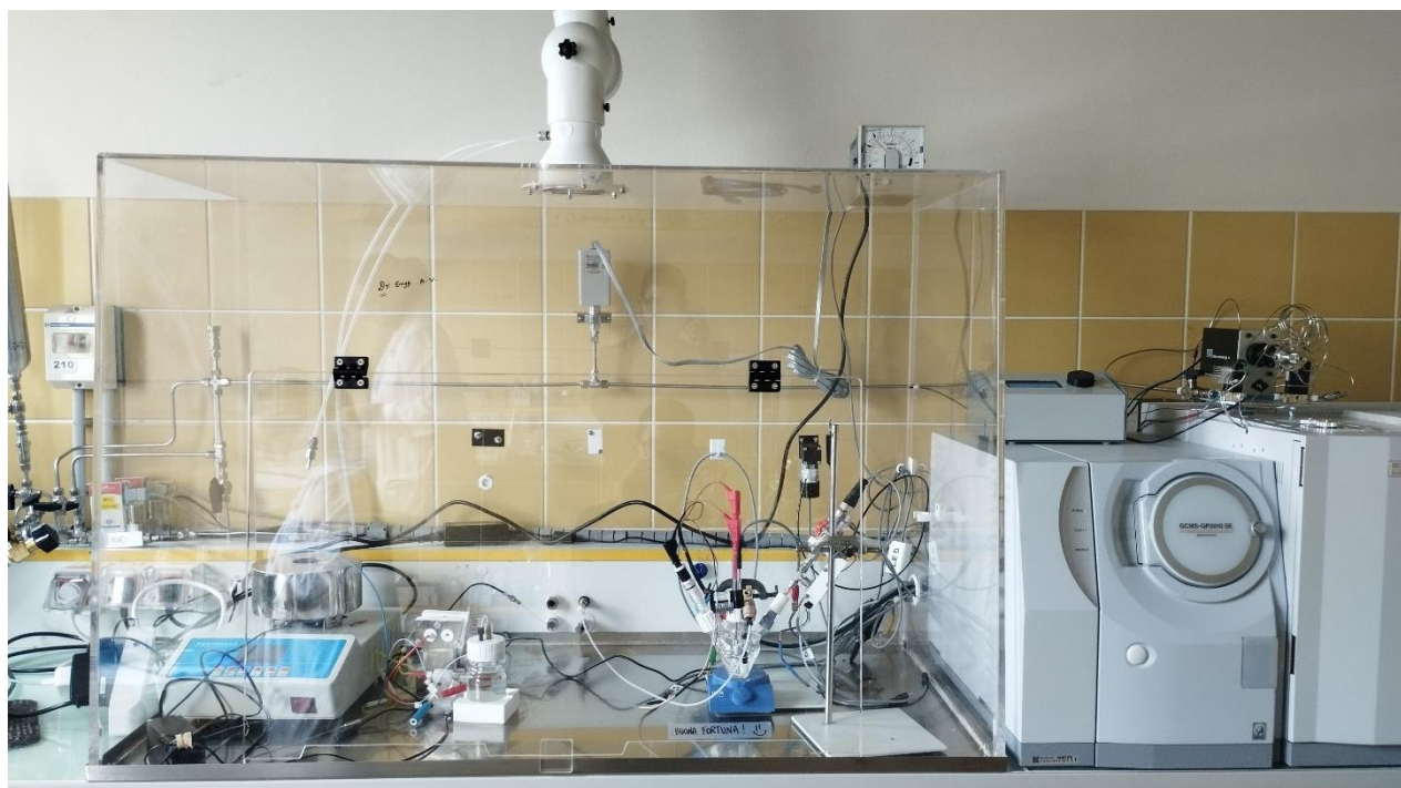
Figure 2-2. Photograph of the electrochemical setup used for the experiments. From left to right, there are mass flow controllers, the electrochemical cell and the GC-MS apparatus.
