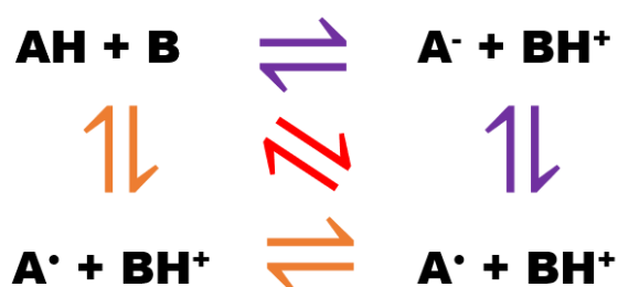
Figure 1-2. Diagram of the three possible pathways for a electron-proton transfer, with the PTEP pathway in purple, the ETPT pathway in orange and the PCET pathway in red.
