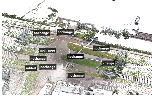
Figure 1.3: Example of a scene from the Change3D dataset with the points of interests and their corresponding labels taken from Ku et al. (2021).
