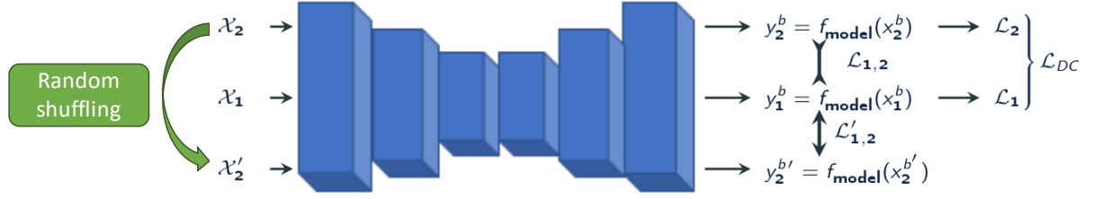
Figure 4.3: Schema of the self-supervised training of the back-bone. The three different losses are alternatively used to modulate the model weights: the deep clustering loss \mathcal{L}_{DC} , the temporal consistency loss \mathcal{L}_{1,2} (with attractive arrows) and the contrastive loss \mathcal{L}'_{1,2} (with repulsive arrows).
