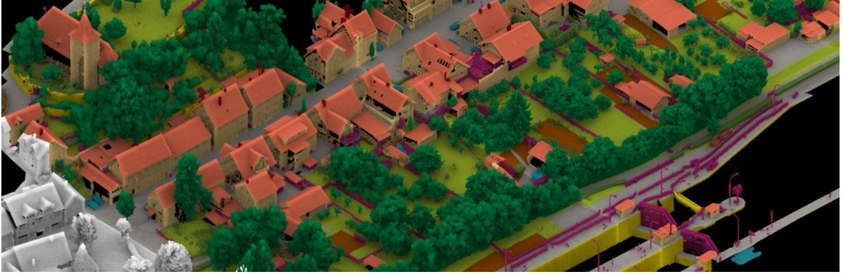
Figure 1.2: Example of H3D dataset (Kölle et al., 2021). The 11 classes are represented in the different colors. Source: Image from (Kölle et al., 2021).
