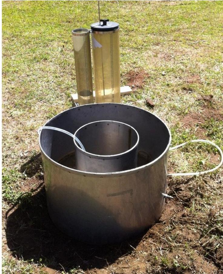
Figure 2.3.3 – Double-ring infiltrometer set-up (from Fatehnia, 2015).
