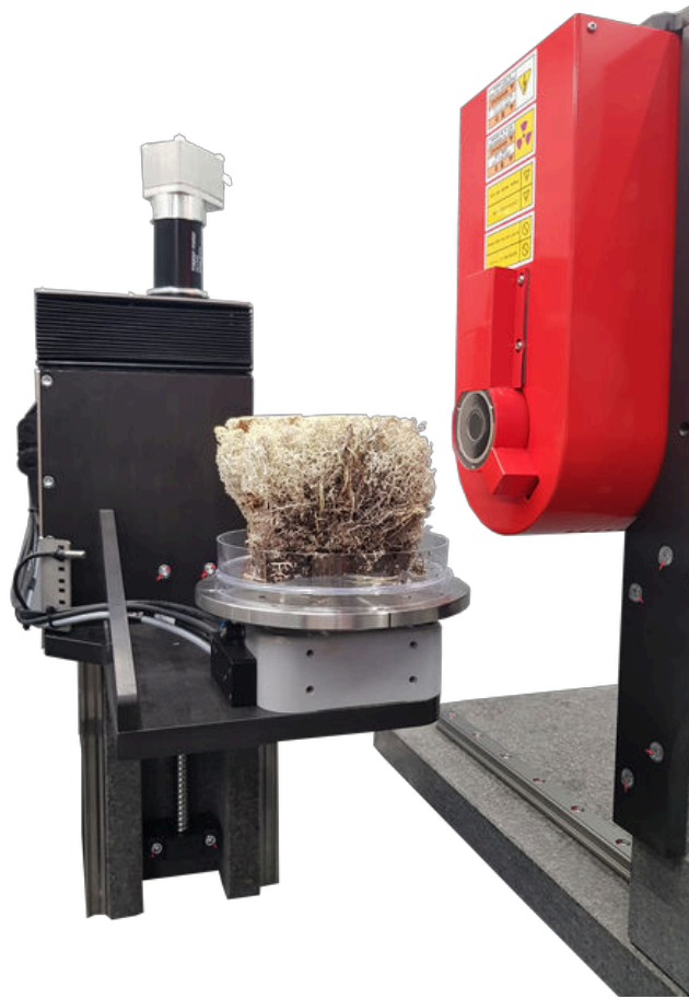
Figure 4.2.2 – Lichen2.1 sample from the Khanymey sample collection being set up for tomography on the CT scan of the Toulouse Institute of Fluid Mechanics. © Yohan Davit, 2018. The sample has been taken outside of its box, which has not been the case for the other acquisitions.
