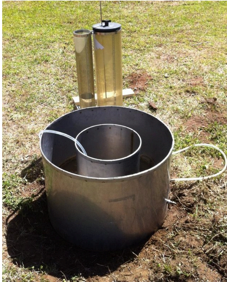
Figure 2.3.3 – Double-ring infiltrometer set-up (from Fatehnia, 2015).
