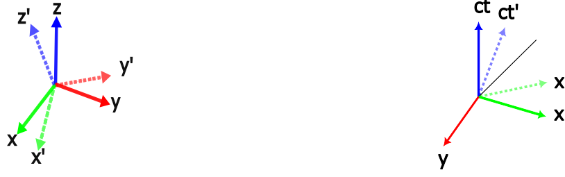
Figure 2.2: Left: ordinary rotation of axes, from unprimed (dashed) to primed (full) axes. Transformations of this type are a subgroup of all Lorentz transformations, where only the spatial coordinates are mixed, i.e. \exists i, j s.t. \Lambda_i^j \neq 0 . Here, the ct -axis is left out intentionally. Right: boost i.e. \exists \mu s.t. \Lambda_0^\mu \neq 0 and \Lambda_\mu^0 \neq 0 , from unprimed (dashed) to primed (full) axes. Here, the z -axis is left out and the diagonal black line represents a light ray. Note that in the primed frame, the ct' - and x' -axis have tilted symmetrically towards the light line, thus leaving the speed of light unchanged in the transformed frame.
