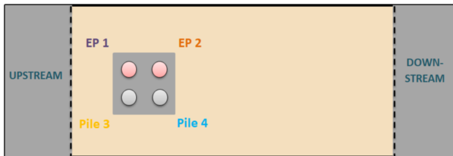
Figure IV. 27 - Schematic representation of piles group for third campaign tests (Top view)
