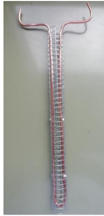
Figure III. 12 - Photo of the reinforcement cage of the energy pile model (Guenneau, 2022)
