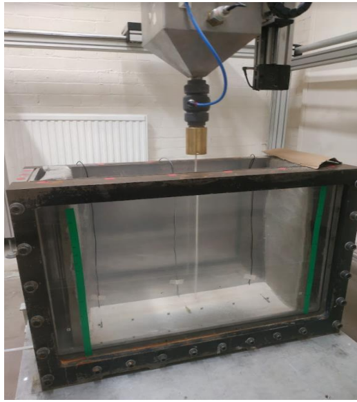
Figure III. 11 - Photography of the box during sand pouring
