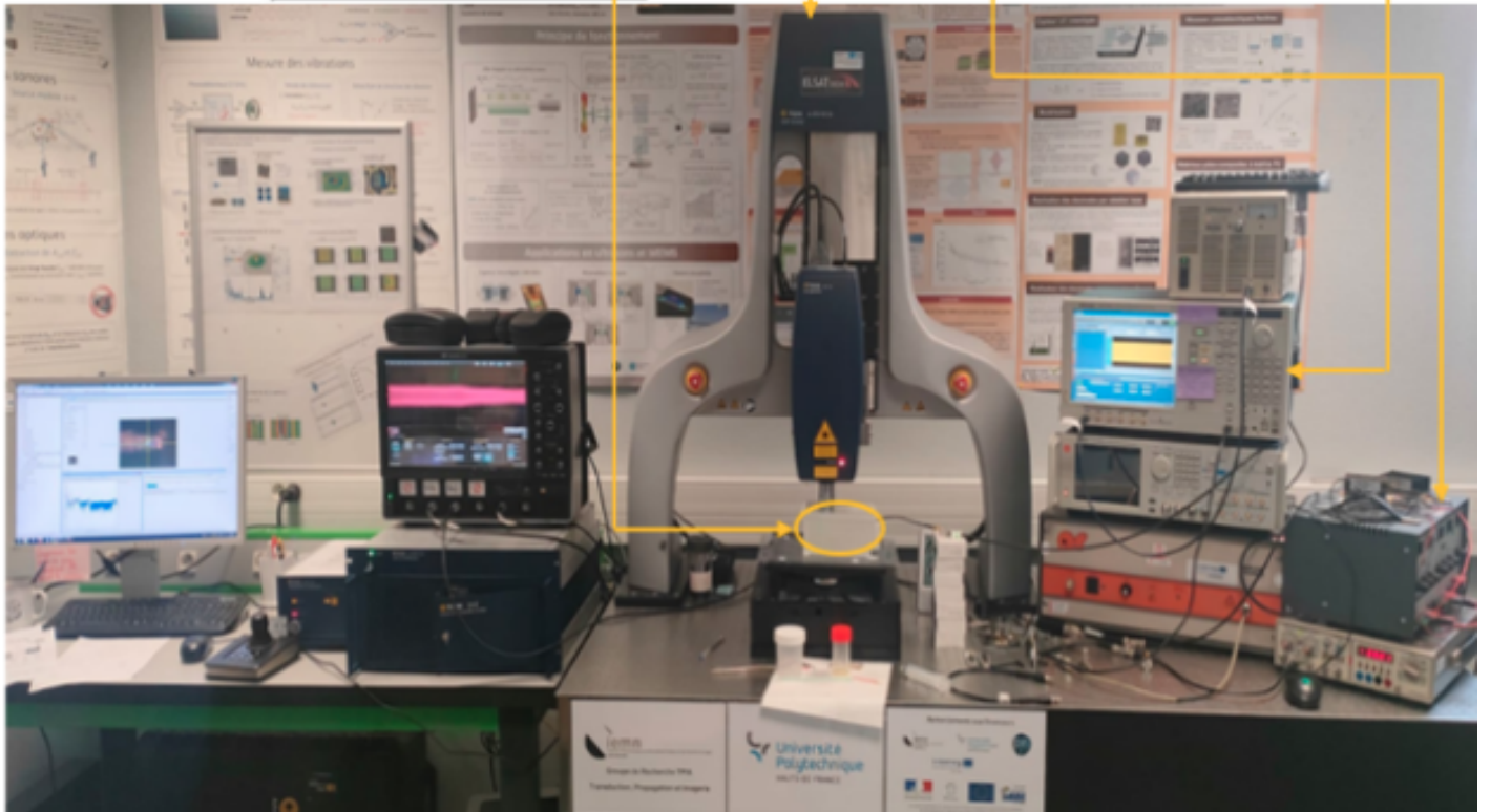
Figure 4.2: Experimental Setup for Investigating Beam Vibrations Using LDV-UHF-120 and MATLAB-Controlled Signal Generation
