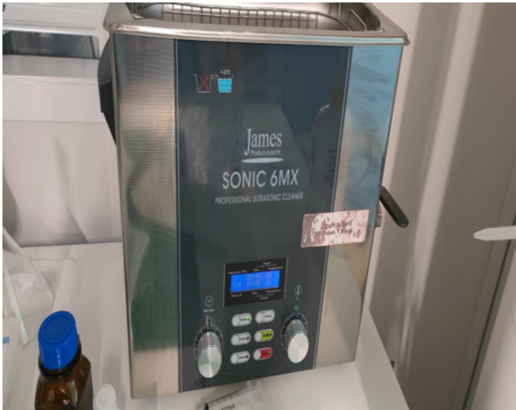
Figure 3.12: Cleaning Samples with Ultrasound Machine
