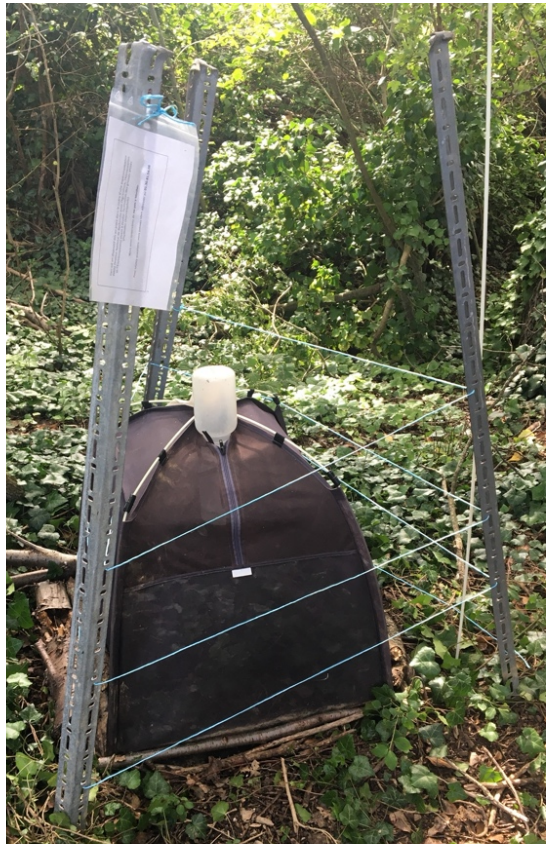
Figure S.2. 1 : Emergence traps (60 x 60 x 60 cm) were placed in three habitats (here, forest edge). They were protected by three iron corners to prevent wild boars' damage.
