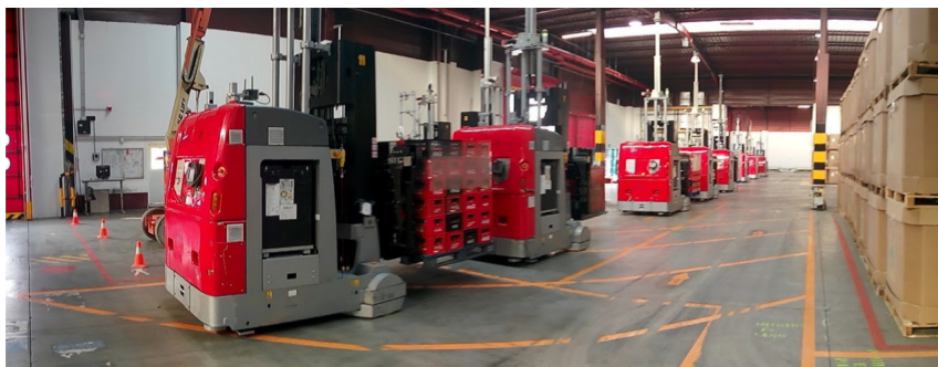
Figure 16: AGVs used for automated goods transport in a warehouse [ Cardarelli et al., 2017 ]
