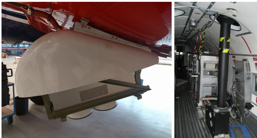
Figure 2.4: Left: MiRAC-A with opened belly pod below the research aircraft Polar 5. Figure adapted from Mech et al. (2019). Right: The AMALi system in zenith-pointing airborne configuration on board the Polar 5 aircraft. Figure adapted from Stachlewska et al. (2010).
