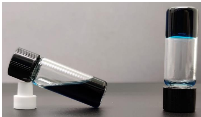
Figure 5.4. Pictures of the “tube inversion” of an n -heptane hot solution and a gel of TbC 6 ( C_m = 10 \text{ mg}\cdot\text{mL}^{-1} ) in 2mL vials (left).
