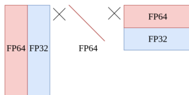
Figure 1.8: A mixed-precision representation of a low-rank matrix, used by Ooi et al.
