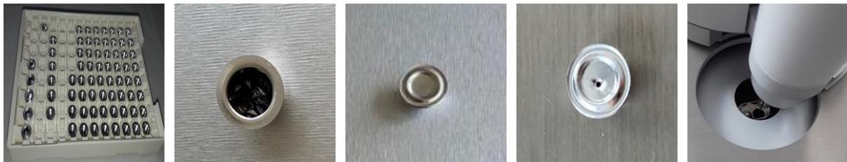
Figure II.14: DSC sample preparation steps
