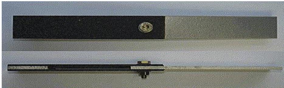
Figure I.16: A typical hybrid joint specimen [5]
