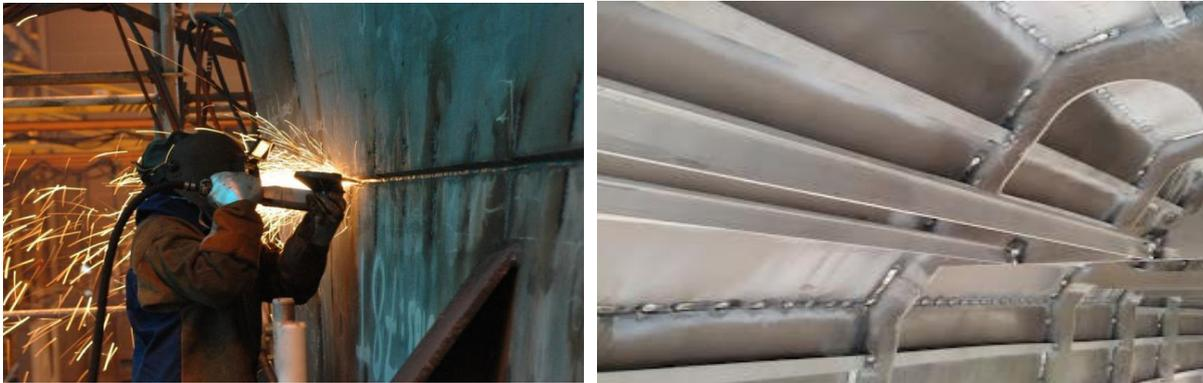
Figure I.5: Welding joint along boat structure [6]
