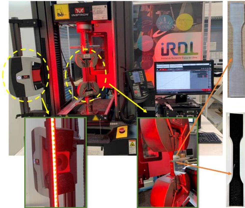
Figure II.18: Tensile test with INSTRON machine
