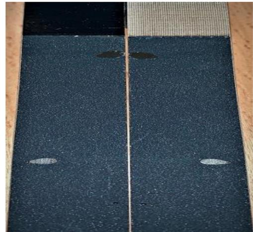
2wt.% GNPs/Adhesive Bonded Aluminum Joint
