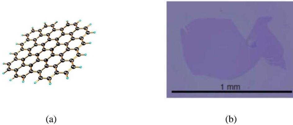
Figure II.4: (a) The structure of graphene (b) Large pieces placed on SiO<sub>2</sub> wafer prepared by "Sellotape method"
