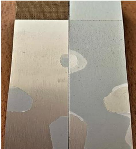
(a) Neat Adhesive Bonded Aluminum Joint
