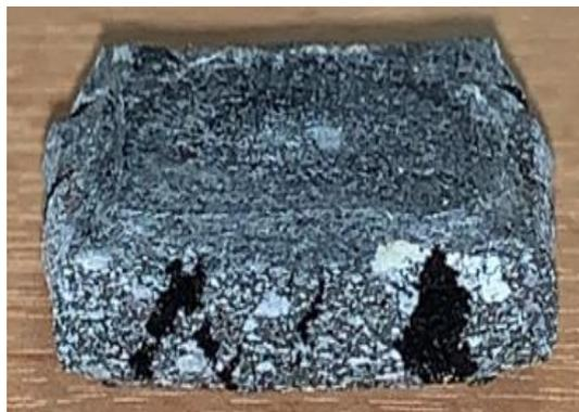
Figure IV.14: Surface Photographic images of CNTs/DGEBA epoxy nanocomposite with different wt.% after compression
