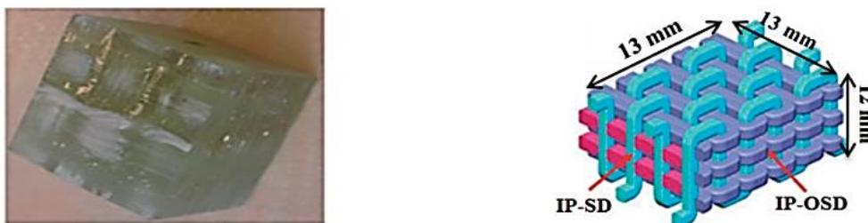
Figure I.28: Specimen of 3D stitched woven composites [106]
