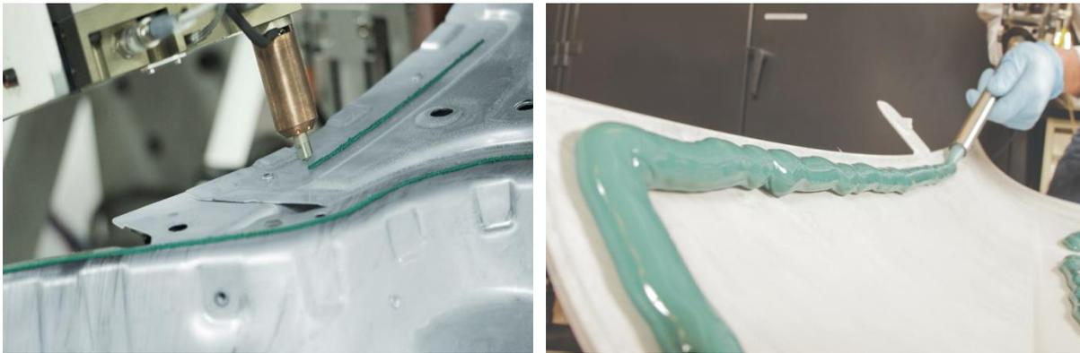
Figure I.8: Adhesively-bonded joint belong boat structure [11]
