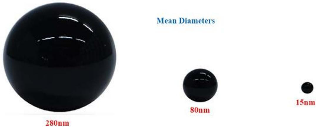
Figure II.7: Carbon Black Particle Dimension Comparison
