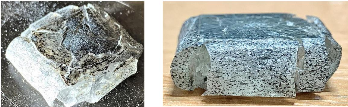
Figure IV.12: Surface Photographic images of neat DGEBA epoxy nanocomposite after compression
