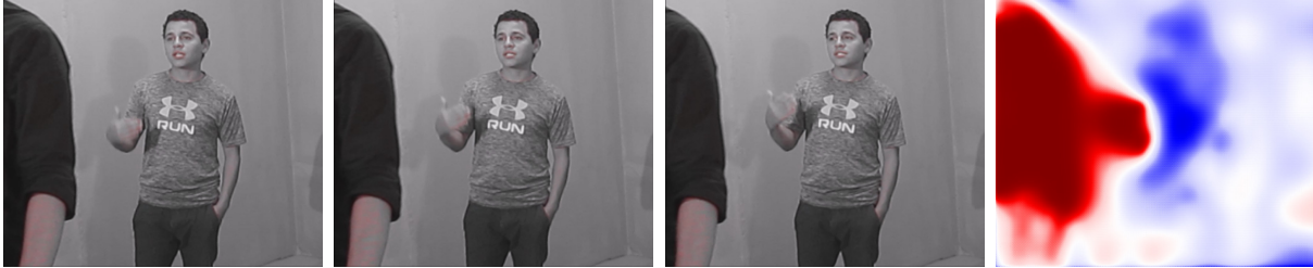
(a) Past reference \hat{\mathbf{x}}_p . (b) Current frame \mathbf{x}_t . (c) Future reference \hat{\mathbf{x}}_f . (d) Mode selection \alpha . blue: skip, red: CNet.
