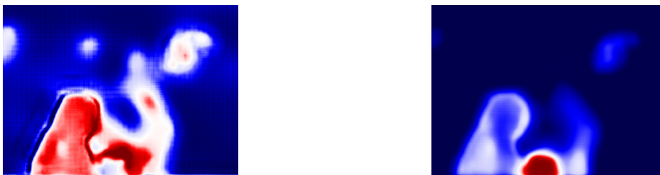
(g) Bidirectional prediction weighting \beta . blue : warp from \hat{\mathbf{x}}_f , red : warp from \hat{\mathbf{x}}_p . (h) Coding mode selection \alpha . blue : skip, red : CNet.
