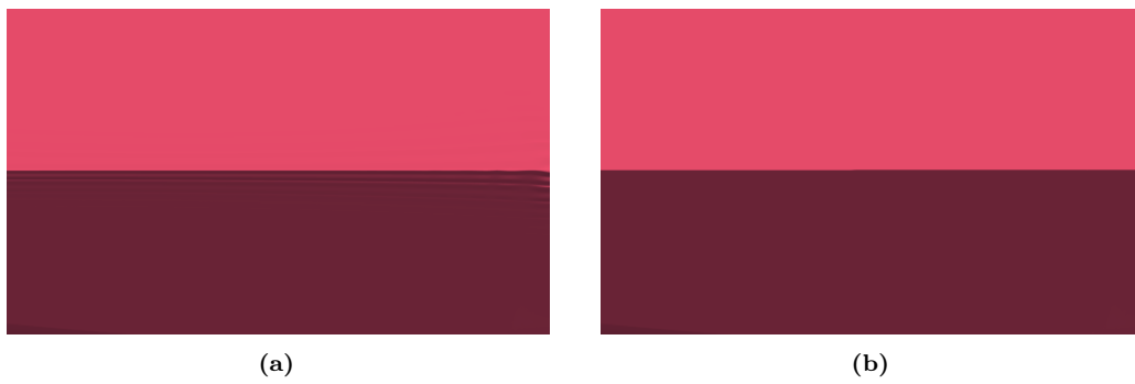
Figure 5.11. Zoom-in of the top edge of the KCS hull model. (a): smoothed edge with consequent oscillations due to the G^1 continuity. (b): sharp edge achieved by imposing C^0 regularity along the sharp edge.
