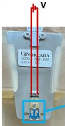
Figure 5.4 (a) Electric biasing system including electric biasing chip, its holder, electric biasing controller, and software. (b) Close-up electric biasing chip and holder. (c) Schematic and microscope image of \text{MAPbI}_3 film on the electric biasing chip.
