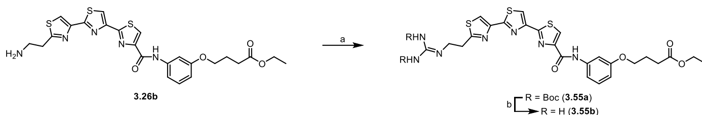
Scheme 20 - Reagents, conditions, and yields: (a) 1,3-Di-Boc-2-(trifluoromethylsulfonyl)guanidine, Et 3 N, DMF, rt, 16h, 97%; (b) 4M HCl in 1,4-dioxane, rt, 30min, 95%.
