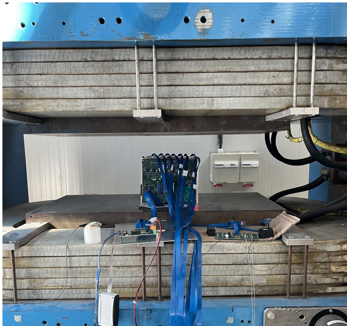
Figure 6.26: Picture of the FEB setup in the MNP17 magnet at CERN.
