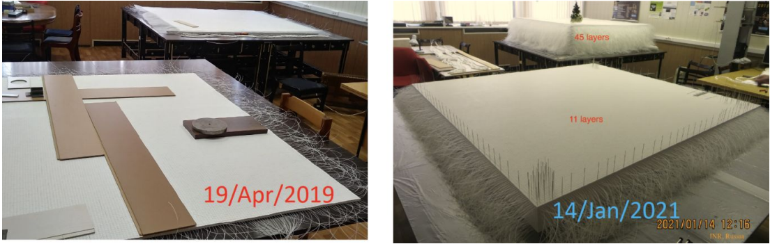
Figure 5.7: Preassembly of the Super-FGD layers with fishing lines. Credits: M. Khabibullin.
