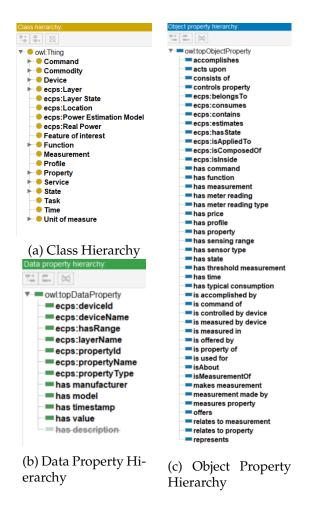
Figure 2.2: SAREF Ontology Extension Implementation in Protégé
