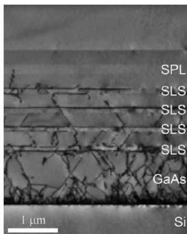
Figure 1.10 Cross-sectional TEM images, displaying the suppression of threading dislocations through the growth of strained superlattice (SPS) and short period superlattices (SPL). Courtesy of [40]
