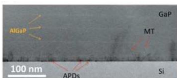
Figure 1.14 STEM-BF images showing the annihilation of most of the APDs at 10nm from the interface. Courtesy of [59]
