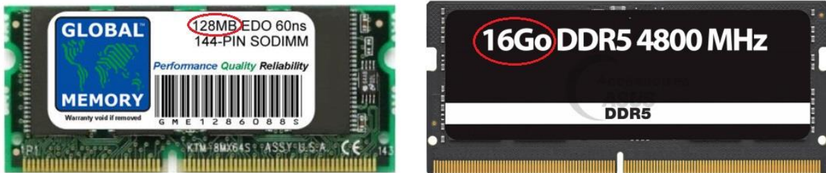
Figure 1 : Random access memory devices (RAM), left: 128 Mo memory capacity produced in 2002 year right: 16 Go memory capacity produced in 2018 (128 times memory capacity in the same device size) 5
