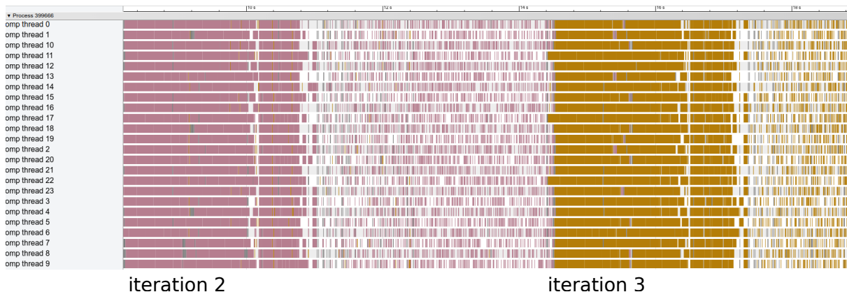
Figure 6.9: LULESH Gantt Chart on 24 Intel(R) Xeon(R) Platinum 8168 CPU @2.70GHz using MPC with -s 384 -i 16 -tel 48 -tnl 48 (left-most point of Fig. 6.8). Distinct colors indicate tasks from distinct iterations.
