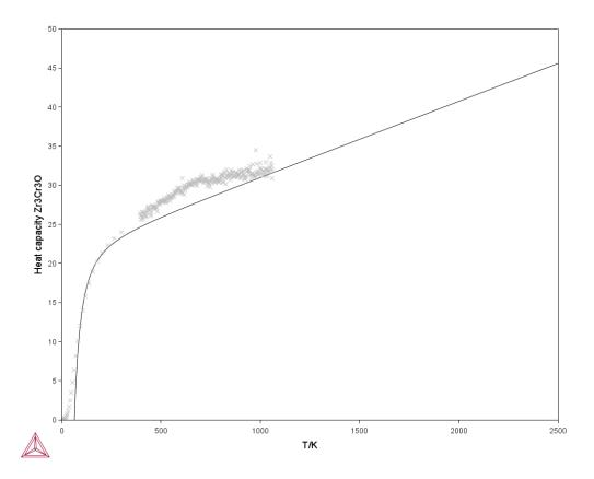
Figure IV-40 Comparison of  $C_p$  calculated from CALPHAD model and experimental points of the ternary phase Zr<sub>3</sub>Cr<sub>3</sub>O
