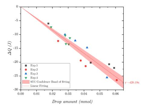
Figure IV-30 Heat change of Zr<sub>3</sub>Cr<sub>3</sub>O versus drop amount in Al bath at 900°C
