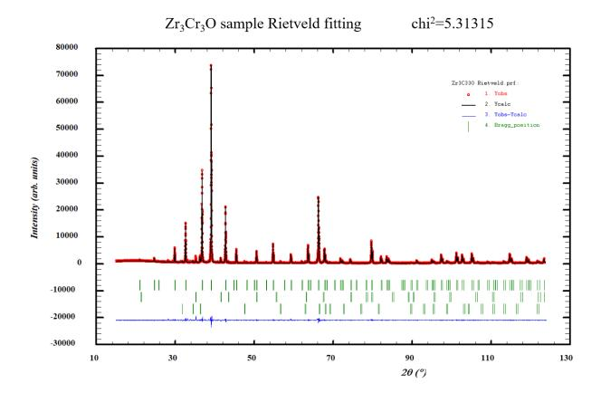
Figure IV-27 Rietveld fitting of the XRD scan of the Zr<sub>3</sub>Cr<sub>3</sub>O sample annealed 3 h at 1400°C (purity 99.3 wt.%).
