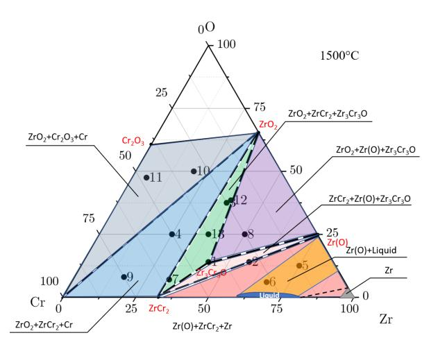
Figure IV-24 Phase relation on the isothermal section at 1500°C of the Zr-Cr-O system. Dashed line is the tentative limit of the liquid + Zr(O) +  $\beta$ -Zr three phase domain.
