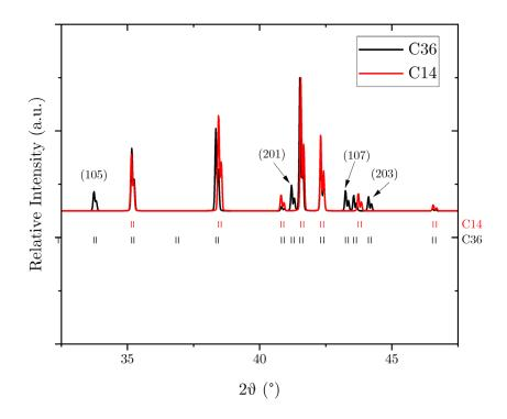
Figure III-3 Comparison of the diffraction patterns of Laves phases C14/C36 of  $ZrCr_2$  in an interval 30~50°. The labeled peaks (105), (201), (107), and (203) are the peaks considered for identification of the C36 phase from C14. The crystallographic information used was detailed in Chapter II.
