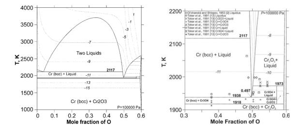
Figure IV-6 Calculated Cr-O phase diagram with oxygen isobars by Povoden *et al.* [27]. The gas phase was not included in the calculation. Enlargement of the calculated Cr-O phase diagram close to the CrO composition, with experimental data and oxygen isobars included.
