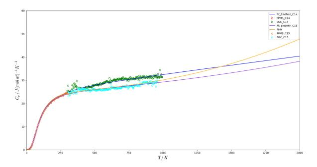
Figure III-29 Comparison of experimental data of  $C_p$  C14/C15 typed ZrCr<sub>2</sub> extended to 2000K, modeling with Equation (III-6) and Neumann-Kopp rule (hcp-Zr and bcc-Cr from data of SGTE).
