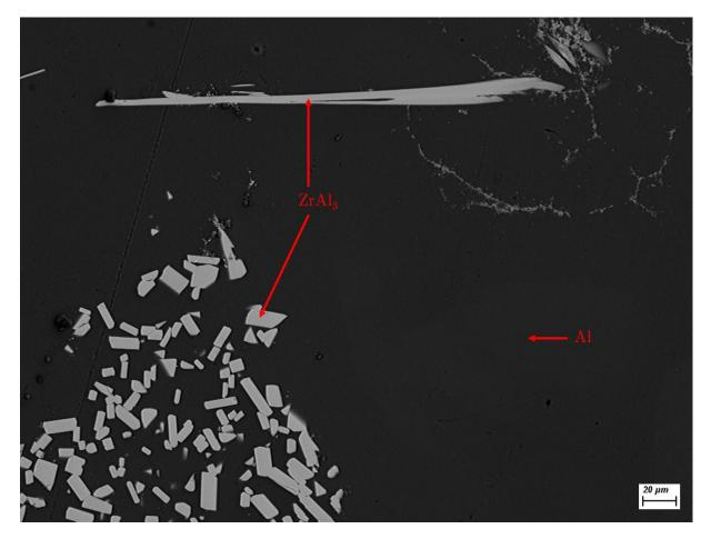
Figure III-25 Ingot of drop solution experiment: ZrCr<sub>2</sub> in solvent Al. The photo was taken by BSE under an accelerating voltage of 20kV, a working distance of 12.3mm
