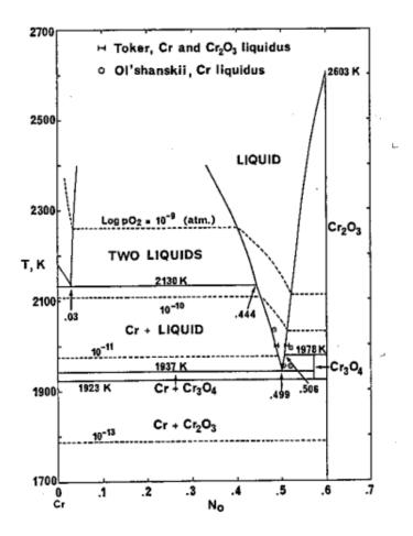
Figure IV-4 Modelled Cr-O binary system of Taylor [23]
