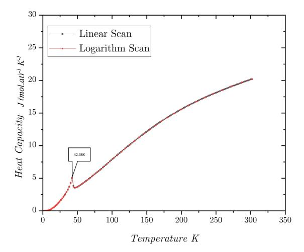
The  $C_p$  at low temperatures was measured by the semi-adiabatic method (PPMS).
