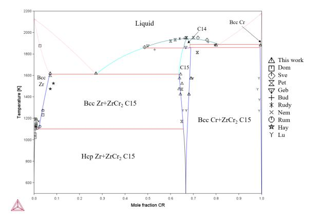
Figure III-30 Calculated phase diagram Zr-Cr of this work. In the legend: Domagala *et al.* [8], Svechnikov and Spektor [12], Petkov *et al.* [15], Gebhardt and Rexer [25], Rudy [14], Nemoshkalenko *et al.* [26], Rumball and Elder [11], Hayes *et al.* [13], Lu *et al.* [5].
