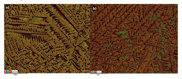
Figure IV-21 SEM images of the sample Zr17Cr75O8 (composition as Zr 17.9% at.; Cr 75.0% at.; O 7.2% at. by EDS). Mapping mode: Pink for O, green for Zr and red for Cr. Images taken under 15kV and magnification x300.
