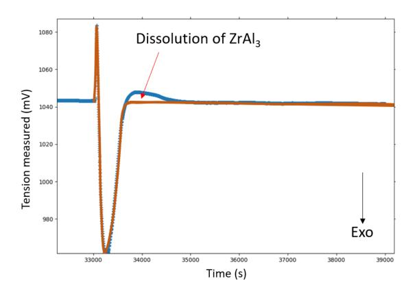
Figure IV-31 Schematic view of two types of thermal curves obtained in the drop solution experiments of  $Zr_3Cr_3O$ . The blue curve corresponds to drops in which the  $ZrAl_3$  formed is subsequently dissolved, while the orange curve corresponds to drops in which the  $ZrAl_3$  formed is not dissolved.
