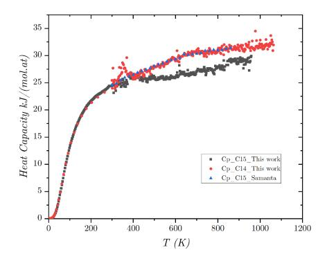
Figure III-28 Comparison of  $C_p$  of C14/C15 obtained in this work and the experimental data of C15 of Samanta and Jain [35].
