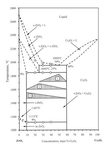
Figure IV-17 Phase diagram of quasi-binary system  $ZrO_2$ - $Cr_2O_3$  by Jerebtsov *et al.* [39]. Triangles show the expected peak areas for 1) eutectic at 1950°C; 2) eutectoid at 1840°C; 3) eutectoid at 1115°C.
