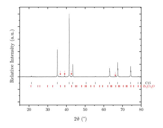
Figure III-13 XRD pattern of a ZrCr<sub>2</sub> sample annealed at 1560°C for 0.5 h (major phase C15) that is slightly oxidized (Zr<sub>3</sub>Cr<sub>3</sub>O). Red arrows point out the weak peaks indicating oxidation.
