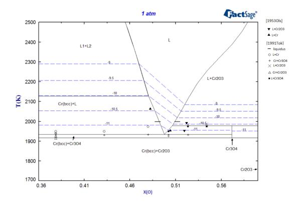
Figure IV-9 Zoom of the Cr-O phase diagram calculated in NUCLEA, with the experimental points [1991Tok]=Toker *et al.* [25], [1953Ols]=Ol'shanskii and Shlepov [29] and the P(O<sub>2</sub>) isobars in atm superimposed
