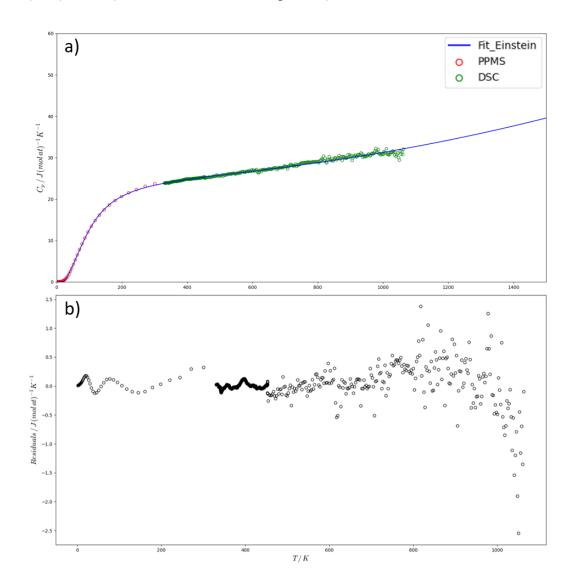
Figure IV-29 Heat capacity of  $Zr_3Cr_3O$  versus temperature. a) Experimental points with the fitting line according to the modified Einstein model in blue. b) difference points between measured and calculated points.
