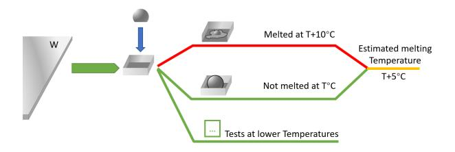
Figure II-1 Schematic view of the step annealing method The melted samples are then examined by SEM and XRD.
