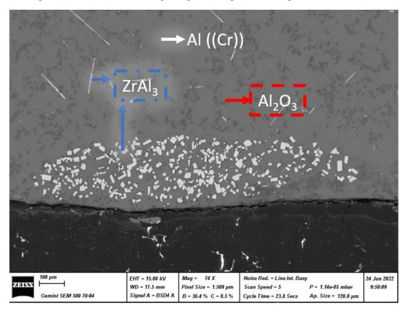
Figure IV-34 Bottom of an ingot exp.2 of drop solution experiment of Zr<sub>3</sub>Cr<sub>3</sub>O
