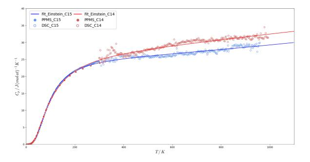
Figure III-26 Experimental C<sub>p</sub> data of ZrCr<sub>2</sub> C14/C15 from 1.8K to 1063K
