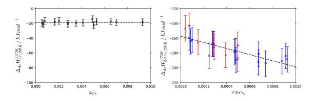
Figure III-22 Linear fitting of drop solution enthalpies for Cr and  $ZrCr_2$ . a) experimental data for Cr, where the dotted line shows the average value; b) experimental data for  $ZrCr_2$  both for the C14 (red triangles) and C15 (blue circles) phases, where the black dashed line is the linear fitting of all the points.
