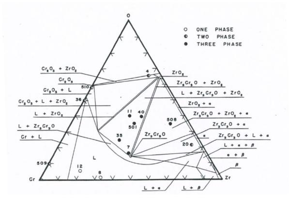
Figure IV-13 Isothermal section of Zr-Cr-O system at 1700°C [1]
