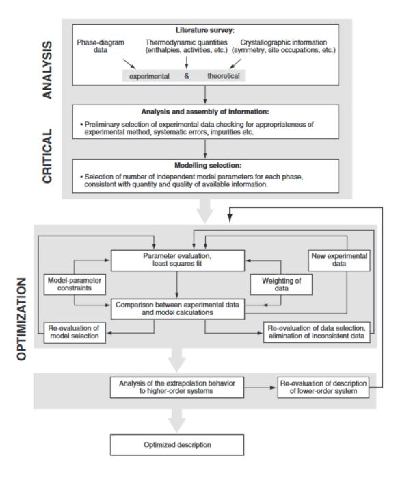
Figure II-6. Principle of the CALPHAD assessment method from Lukas et al. [37]
