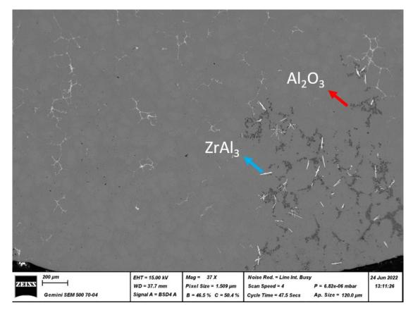
Figure IV-33 Bottom of an ingot exp.1 of drop solution experiment of Zr<sub>3</sub>Cr<sub>3</sub>O
