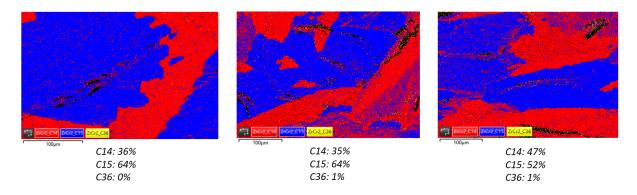
Figure III-10 EBSD maps of  $ZrCr_2$  specimens annealed 1 h at 1125°C. C14: red zones, C15: blue zone, C36: yellow zone. The phase fraction of each polymorph detected is noted below each figure in % at.
