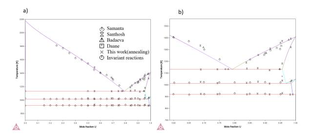
Figure V-10 Assessed phase diagram of the U-Cr binary system in this work. a) Global view; b) Zoomed diagram in the U-rich side.
