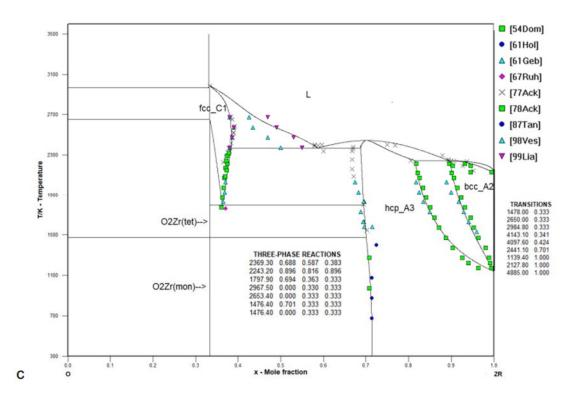
Figure IV-3 Zr-O binary system modeled by Chevalier et al. [7] retained in this work
