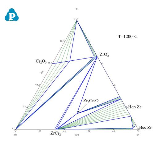
Figure IV-37 Isothermal section of the Zr-Cr-O ternary system at 1200°C
