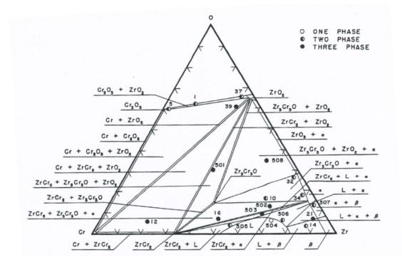
Figure IV-12 Isothermal section of Zr-Cr-O system at 1500°C [1]
