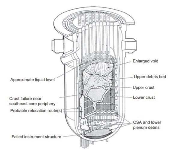
Figure I-2 Hypothesized core damage configuration at 226 minutes [3]
