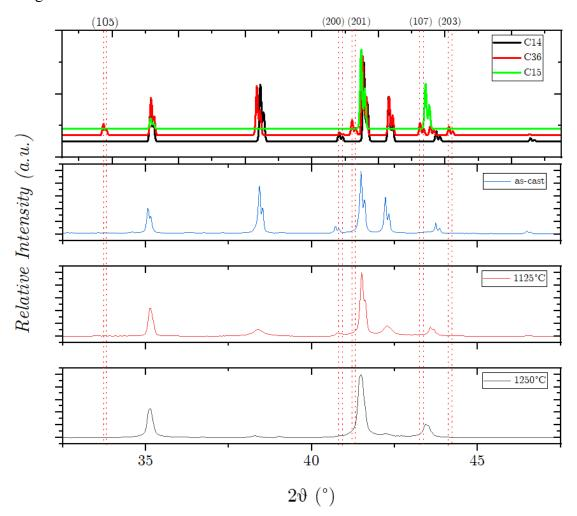
Figure III-11. 30°-50° range of XRD patterns of samples at the as-cast state or annealed 1h at 1125°C, or 1250°C. The top of the figure shows a comparison of the calculated diffraction peaks of the C14, C36 and C15 structures. Crystallographic parameters used in the calculations are detailed in Chapter II. The vertical red dotted lines and Miller indices show the diffraction peaks to identify C36 from C14.
