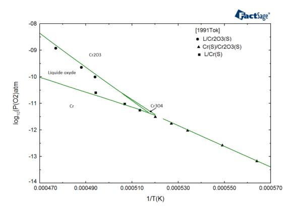
Figure IV-10 Oxygen partial pressure calculated for two-phase equilibria, compared with experimental values from Toker *et al.* [25]
