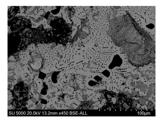
Figure V-19 SEM-BSE image of sample U75Cr5O25
