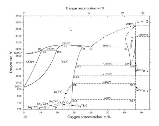
Figure IV-1 Phase diagram of Zr-O binary system [2]
