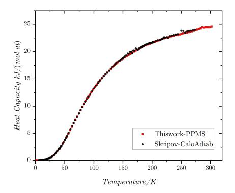
Figure III-27 Comparison of  $C_p$  of Laves phase C15 of ZrCr<sub>2</sub> at low temperatures (1.8K to 300K) obtained by PPMS (this work) and by adiabatic calorimeter (Skripov *et al.* [34]).
