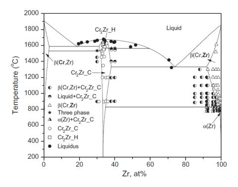
Figure III-6 Phase diagram published by Yang et al. [6]
