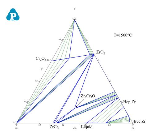
Figure IV-38 Isothermal section of the Zr-Cr-O ternary system at 1500°C
