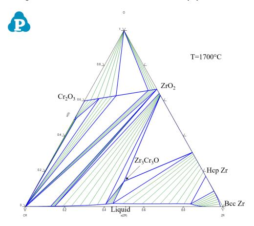
Figure IV-39 Isothermal section of the Zr-Cr-O ternary system at 1700°C
