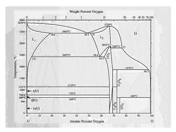
Figure V-11 Assessed phase diagram of the U-O system [16]
