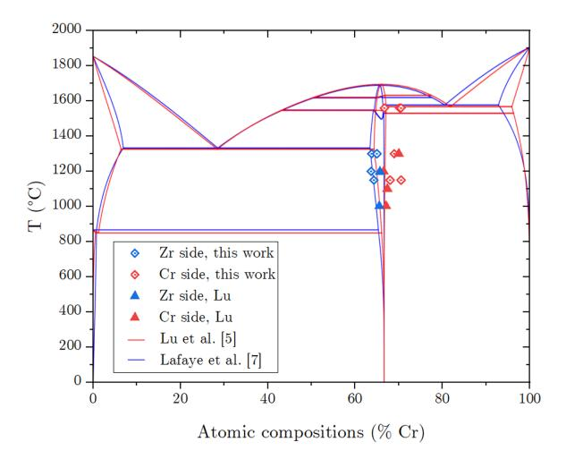
Figure III-15 Measurements of solubility limits on the Zr-rich (blue points) and Cr-rich (red points) sides of  $ZrCr_2$  superimposed on the phase diagrams of Lafaye *et al.* [7] (blue lines) and Lu *et al.* [5] (red lines)
