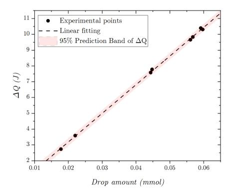
Figure IV-35 Drop heating measurements of  $Zr_3Cr_3O$  at 900°C and linear fitting of the obtained values
