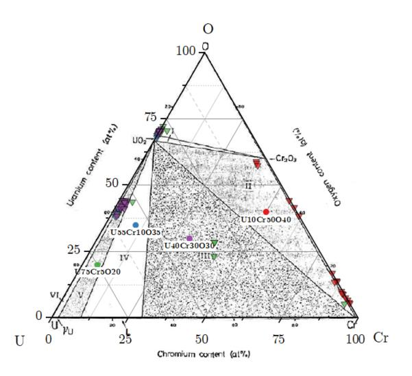
Figure V-13 Prepared samples and EDS measured compositions (%at.) in different areas of each sample reported in the phase diagram of Yamanaka *et al.* [28]. In the figure, dots are prepared compositions of each sample and triangles are measurements by EDS. Symbols with the same color are for the same sample.
