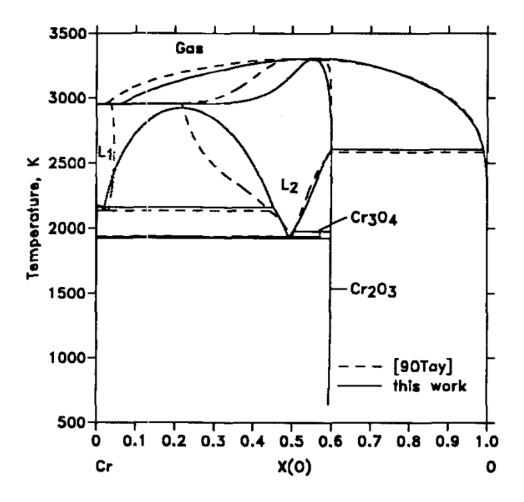
Figure IV-5 Phase diagram of Cr-O system [24] compared to [23]
