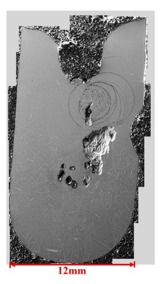
Figure III-24 Vertical cross-section of the solidified ingot of drop solution experiment: Cr in solvent Al. The image is a stitching of 40 photos taken by SEM-BSE. Two phases were identified in the ingot: the white needle-like phase is Al<sub>7</sub>Cr and the grey background is Al.
