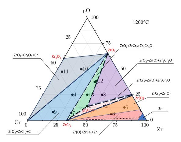
Figure IV-23 Phase relation on the isothermal section at 1200°C of the Zr-Cr-O system. Dashed lines are tentative limits of the  $Zr(O) + ZrCr_2 + \beta$ -Zr three phase domain.
