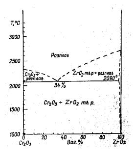
Figure IV-15 Phase diagram of the system ZrO<sub>2</sub>-Cr<sub>2</sub>O<sub>3</sub> reported by Berezhenoi and Gulko [34]
