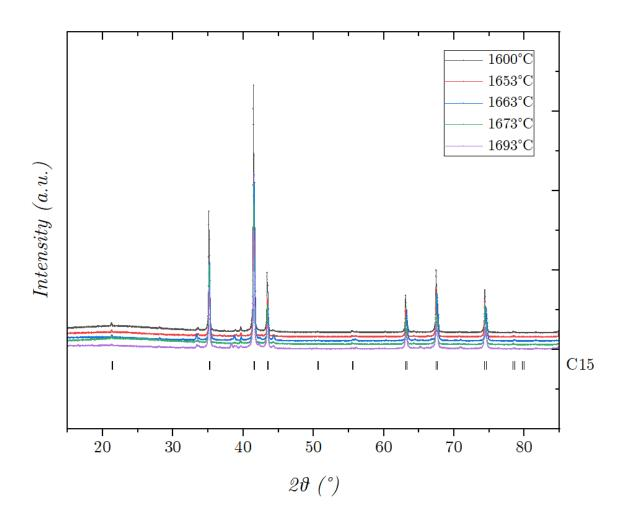
Figure III-17 XRD patterns of step annealing ZrCr<sub>2</sub> samples at different temperatures
