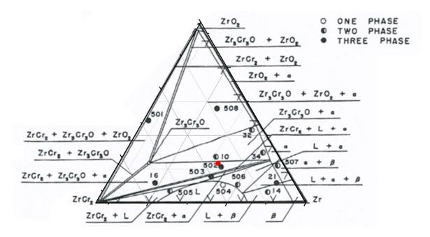
Figure IV-25 Partial phase diagram in the range of Zr-ZrO<sub>2</sub>-ZrCr<sub>2</sub> at 1500°C [1]. Red point: sample 6 (Zr67Cr27O6).
