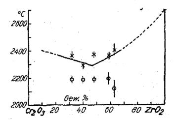
Figure IV-14 Phase diagram of the system ZrO<sub>2</sub>-Cr<sub>2</sub>O<sub>3</sub> reported by Wartenberg and Werth [33]
