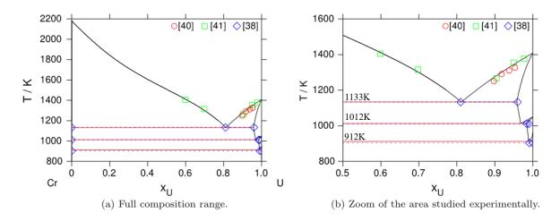
Figure V-2 Assessed U-Cr phase diagram by Berche *et al.* [9]. In the legend at the top right of the graphs, [38] is the publication of Venkatraman *et al.* [1], [40] is the publication of Daane *et al.* [3], [41] is the publication of Badaeva and Kuznetsova [4].
