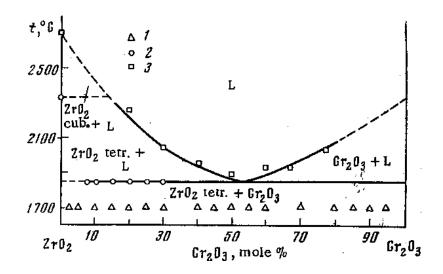
Figure IV-16 Phase diagram of the system  $ZrO_2$ - $Cr_2O_3$  constructed by Lopato *et al.* [35]; (1)= annealing and quenching, (2) = DTA method, (3) = improved DTA method
