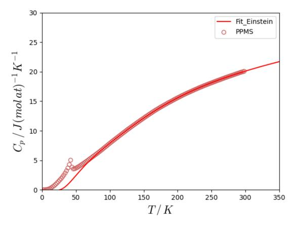
Figure V-22 Fitted  $C_p$  of UCrO<sub>4</sub> with modified Einstein model
