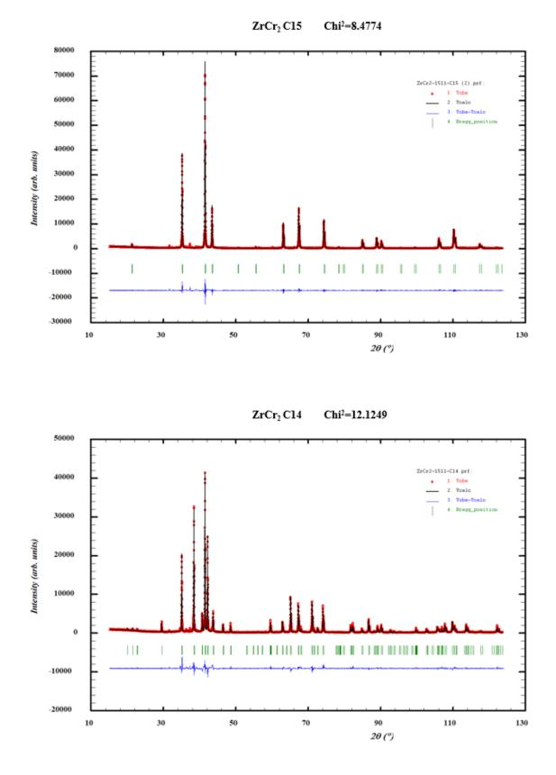
Figure III-12 Rietveld fitting of the XRD patterns of  $ZrCr_2$  C15 (above) and C14 (below)  $ZrCr_2$  polymorphs
