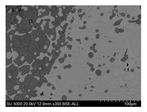
Figure V-16 SEM-BSE micrograph of sample U40Cr30O30
