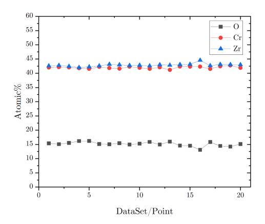
Figure IV-26 EPMA results of Zr<sub>3</sub>Cr<sub>3</sub>O samples
