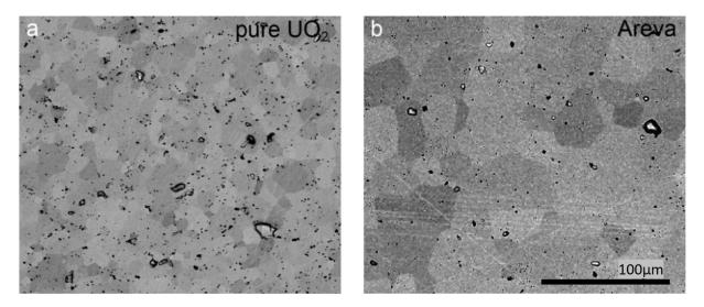
Figure I-5 BSE images of sintered pellets. a) pure  $UO_2$  sintered at 1700°C and oxygen potential -420kJ/mol for 10h; b) Cr-doped  $UO_2$  sample, sintering conditions unknown [36]. The two photos are at the same scale.
