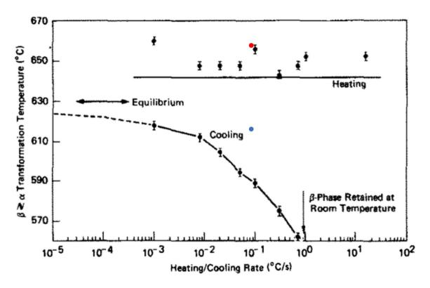
Figure V-9 The  $T_{\alpha \Rightarrow \beta}^{U,Cr}$  temperatures measured in different heating or cooling rates by Chapman [5]. The red and blue points in the figure are our measurements of heating or cooling, respectively
