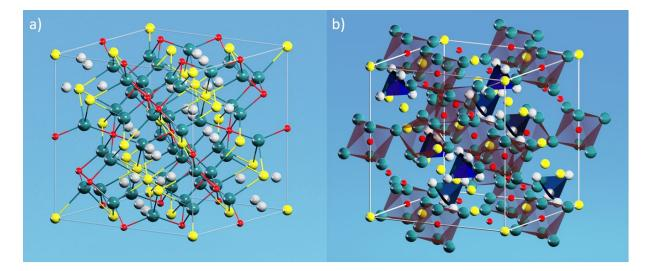
Figure IV-28 a) Perspective view of the crystal structure of  $Zr_3Cr_3O$  phase. b) Perspective view of  $Zr_3Cr_3O$  enlighten the Zr6O polyhedral details. Red spheres stand for oxygen atoms; green spheres stand for Zr atoms; yellow spheres stand for Cr atoms in 16c positions; white spheres stand for Cr in 32e positions.
