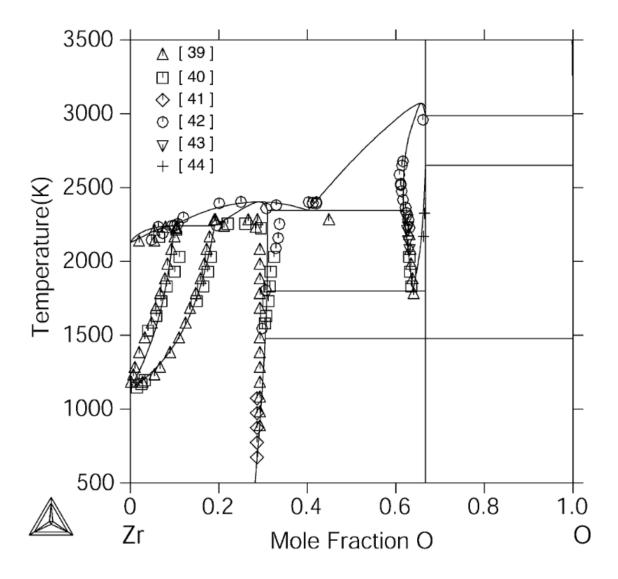
Figure IV-2 Assessed the Zr-O binary system of Wang [8] with experimental data [39]=Domagala and McPherson [16], [40]= Gebhardt *et al.* [17], 41=Holmberg *et al.* [18], [42] Ackermann *et al.* [19], [43] R.J. Ackermann *et al.* [20], [44]=Rauh and Garg [21] superimposed.
