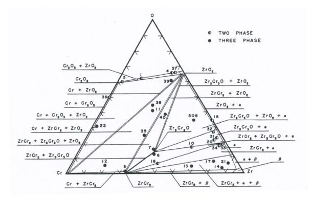
Figure IV-11 Isothermal section of Zr-Cr-O system at 1200°C [1]
