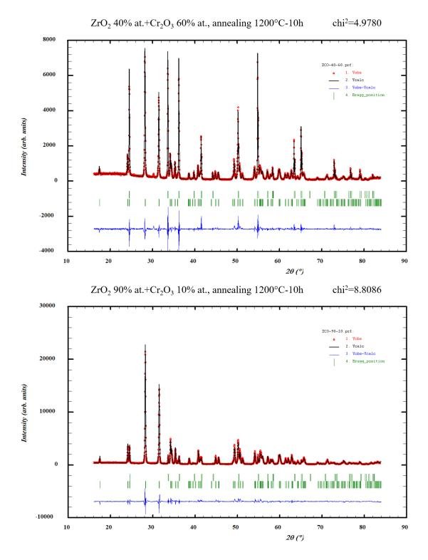
Figure IV-18 Rietveld plots of two samples (above: 40  $ZrO_2\%$  at. 60  $Cr_2O_3$  %at., below: 90  $ZrO_2\%$  at. 10  $Cr_2O_3$  % at.: annealed at 1200°C for 10h.
