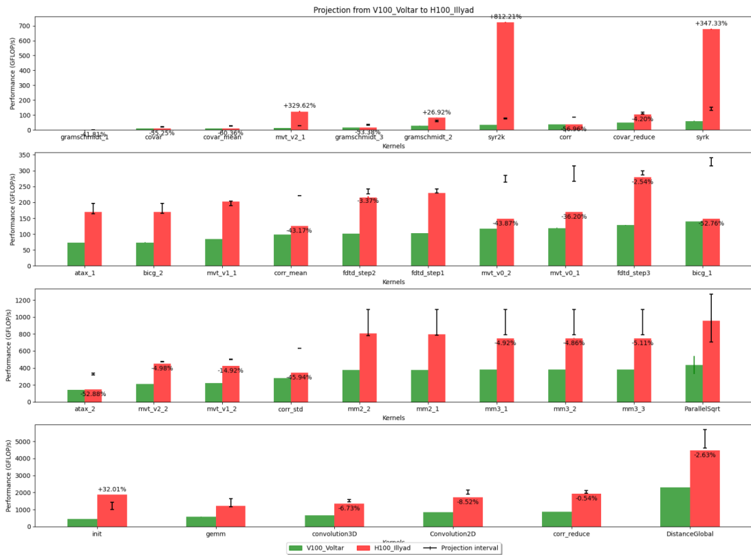
Figure 7.6: N100 \rightarrow H100 projection results on UVMBench benchmark suite, courtesy of L. Van Lanker
