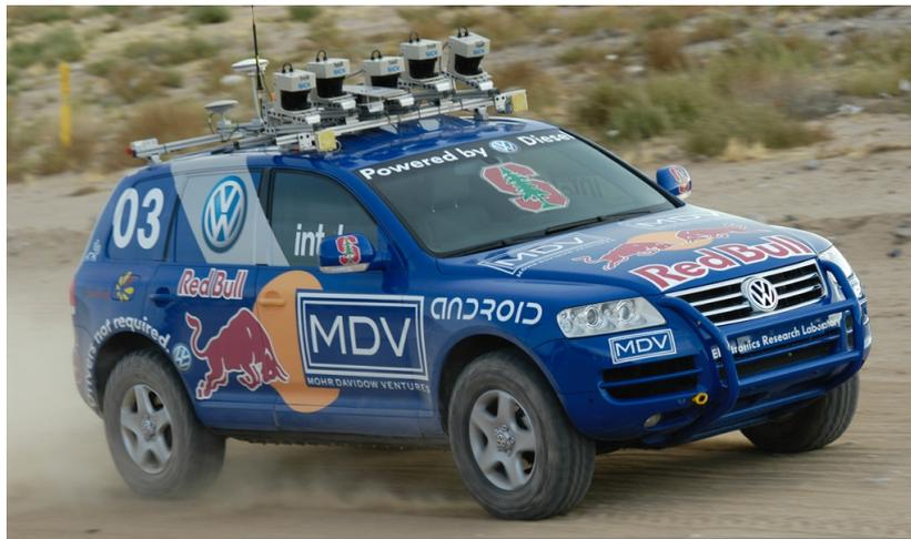
Figure 2: DARPA challenge winning car from Stanford, which was the first to integrate machine learning models to drive. Source: herox.com
