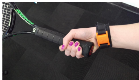
Figure 1.9 – Placement of an inertial measurement unit on the wrist for external load quantification [2].
