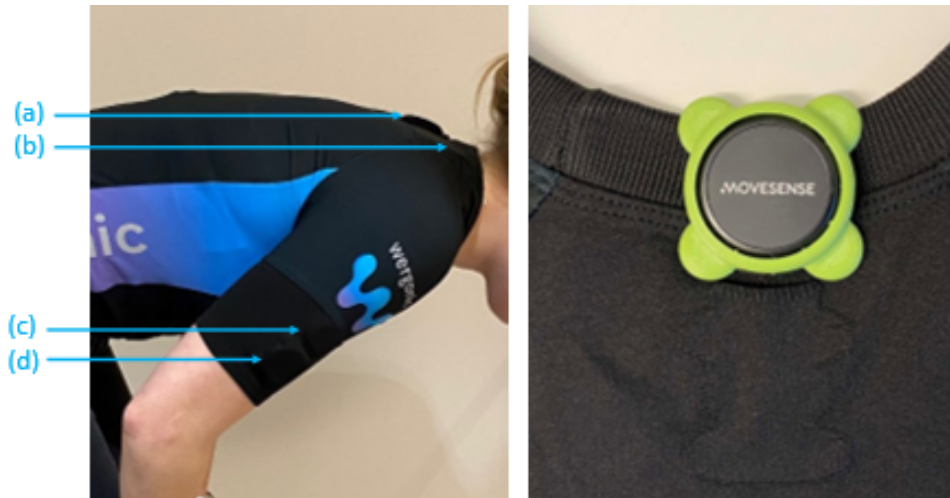
Figure 5.1 – To the left: the two sensor setups showing (a) the trunk sensor in the shirt, (b) the trunk sensor on the skin, (c) the right upper arm sensor on the skin, and (d) the right upper arm sensor in the shirt. To the right: the Wergonic T-shirt pocket and the matching sensor case.
