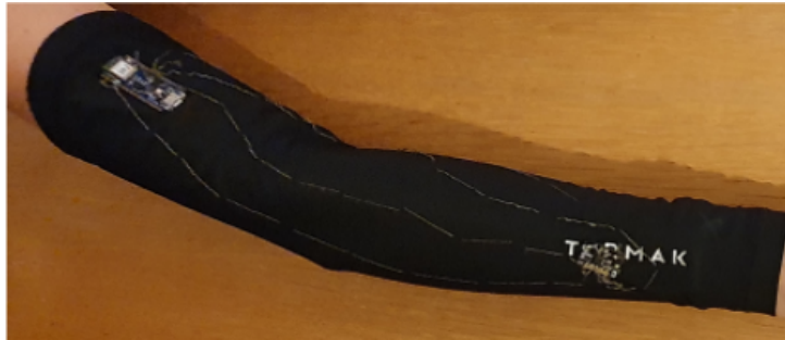
Figure 5.12 – Components integrated in a sleeve using conductive yarns.
